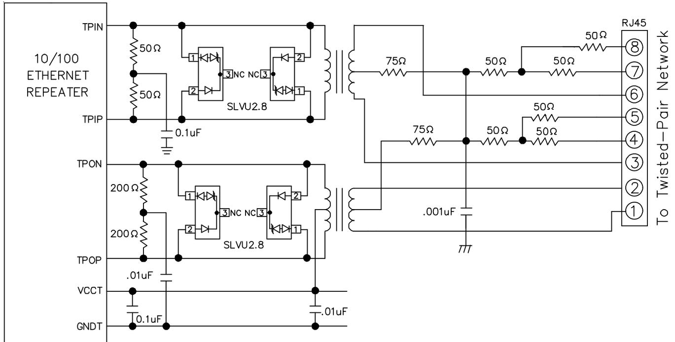
**10/100 Ethernet "Enhanced" Lightning Protection Circuit**
