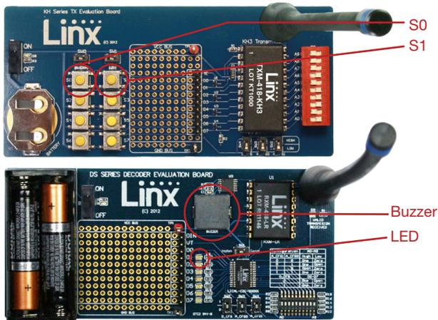
Push S0 to activate buzzer and push S1 to turn on the LED.
