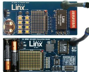
Install batteries and an antenna on each board.
