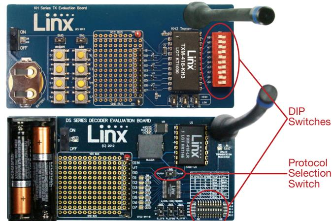
Ensure the DIP Switches are set the same. All switches on and all switches off are not valid settings. At least 1 must be different.
