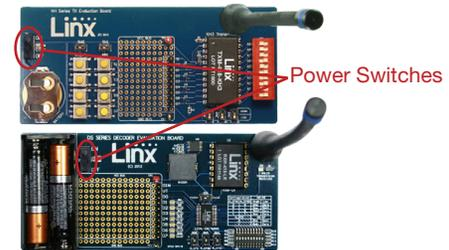
Turn on the power switch on each board.
