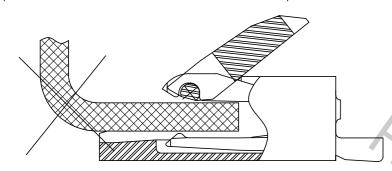
5. When inserting an FPC, do not use the method shown in the photo on the left below where the corner of the FPC is inserted first and then slid sideways, the FPC's corner can deform the terminal's contacts. Always insert the FPC parallel to the board as shown in the photo on the right below.
