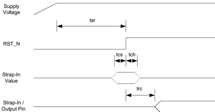
Figure 7. Reset Timing
