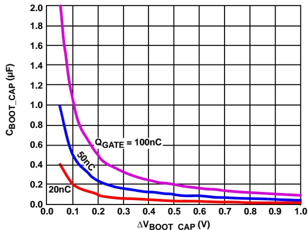
FIGURE 5. BOOTSTRAP CAPACITANCE vs BOOT RIPPLE VOLTAGE
