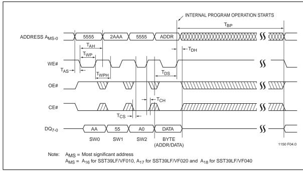
Figure 5: WE# Controlled Program Cycle Timing Diagram
