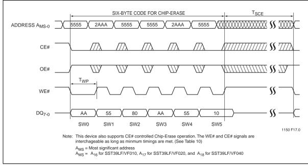
Figure 10:WE# Controlled Chip-Erase Timing Diagram
