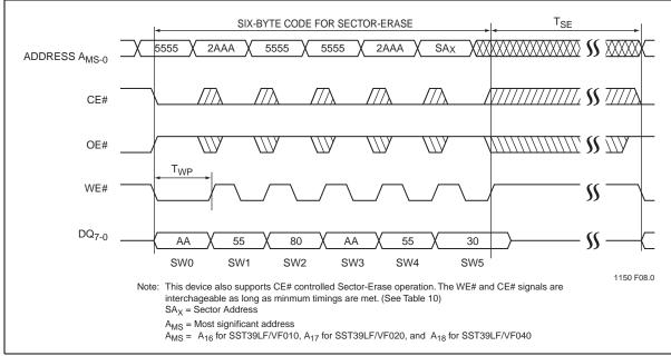
**Figure 9:** WE# Controlled Sector-Erase Timing Diagram
