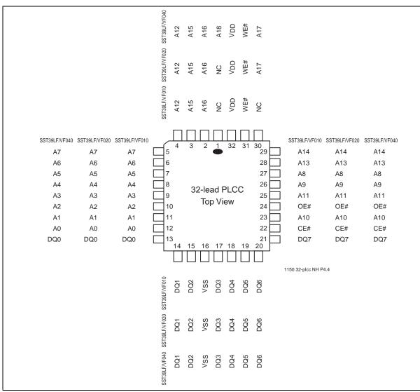
Figure 2: Pin Assignments for 32-lead PLCC
