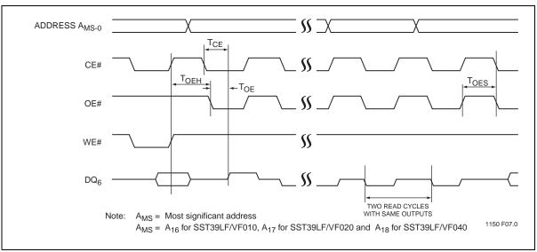
Figure 8: Toggle Bit Timing Diagram
