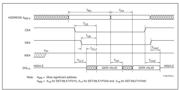
Figure 4: Read Cycle Timing Diagram
