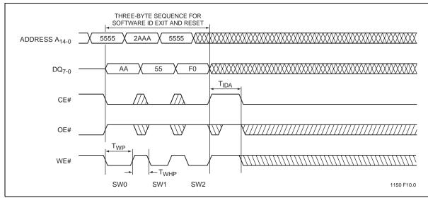
Figure 12:Software ID Exit and Reset
