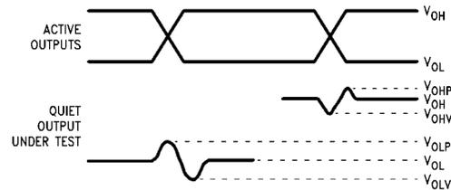
$V_{OHV}$  and  $V_{OLP}$  are measured with respect to ground reference.
