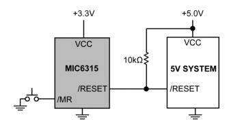
Figure 1. MIC6315 as Used in a Multiple Supply System
