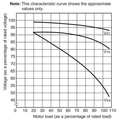
**Note:** For phase loss of phase R. V<sub>st</sub>, V<sub>tr</sub>, and V<sub>rs</sub> indicate the motor terminal voltage at phase loss.
