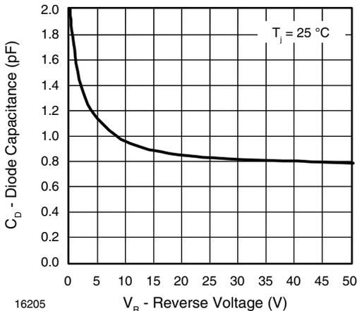
Fig. 2 - Diode Capacitance vs. Reverse Voltage
