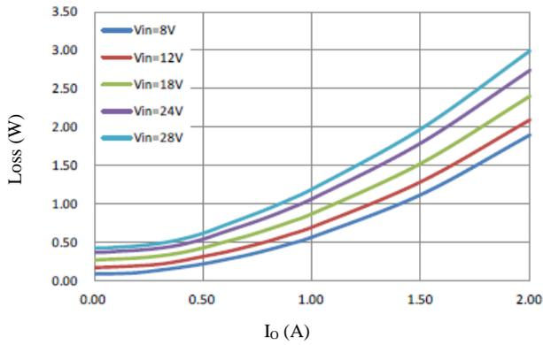
Figure 12-3. Internal Loss
