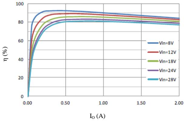
Figure 12-1. Efficiency Characteristics
