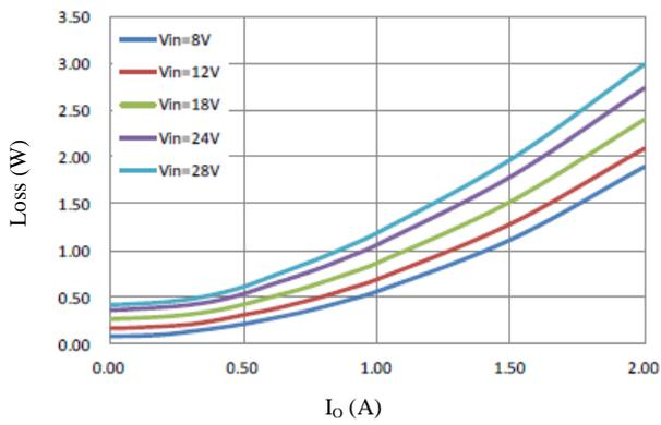
Figure 12-11. Internal Loss
