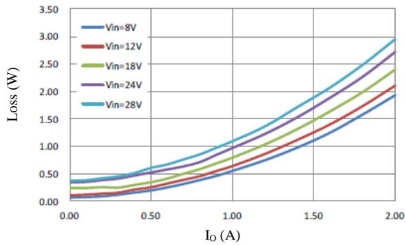
Figure 12-7. Internal Loss
