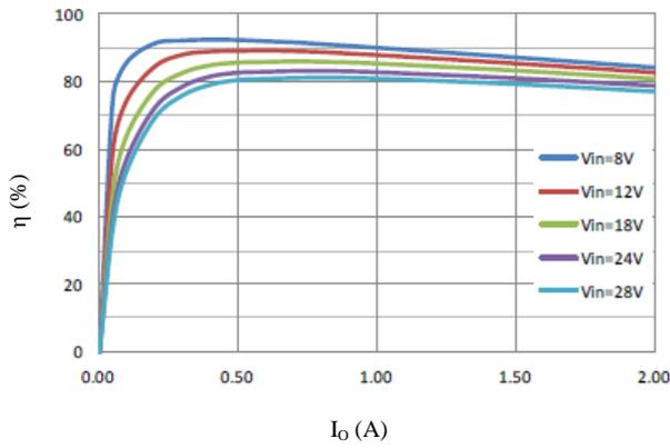
Figure 12-9. Efficiency Characteristics
