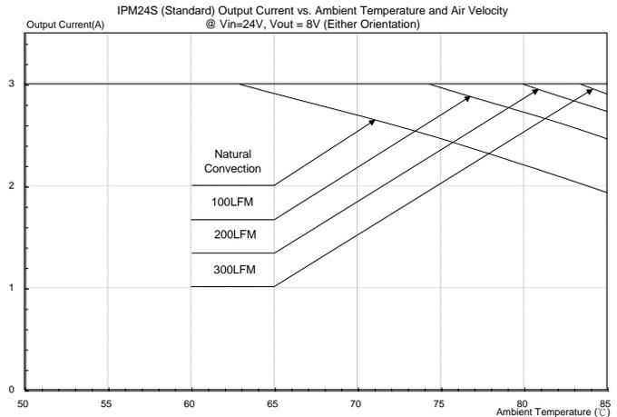
**Figure 26:** Output current vs. ambient temperature and air velocity
