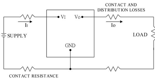
**Figure 17:** Output voltage and efficiency measurement test setup
