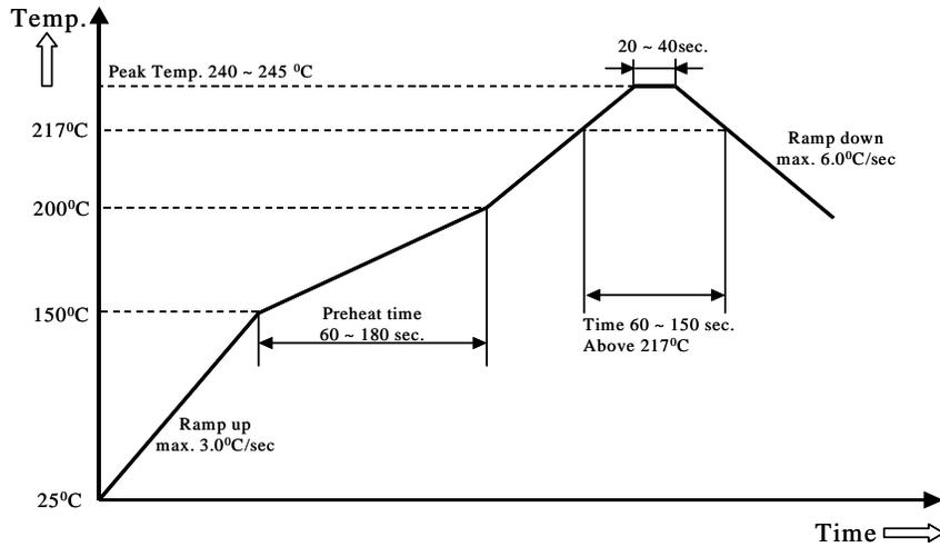
Note: All temperature refers to topside of the package, measured on the package body surface.
