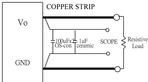
Note: Use a 100µF x 2 OS-con and 1µF capacitor. Scope measurement should be made using a BNC connector.
