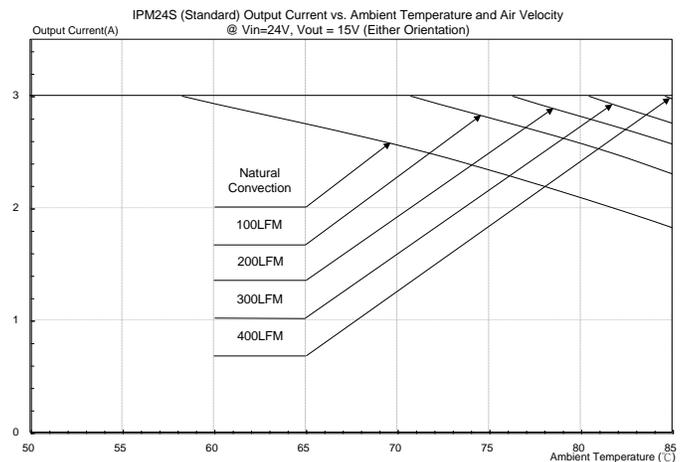
**Figure 27:** Output current vs. ambient temperature and air velocity
