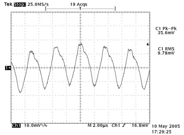
**Figure 4:** Output ripple & noise at 36Vin, 15.0V/3A out
