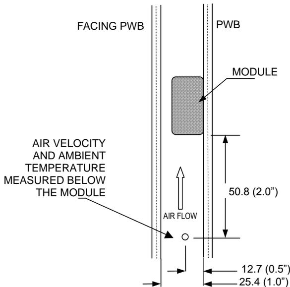
**Note:** Figure dimensions are in millimeters and (inches)
