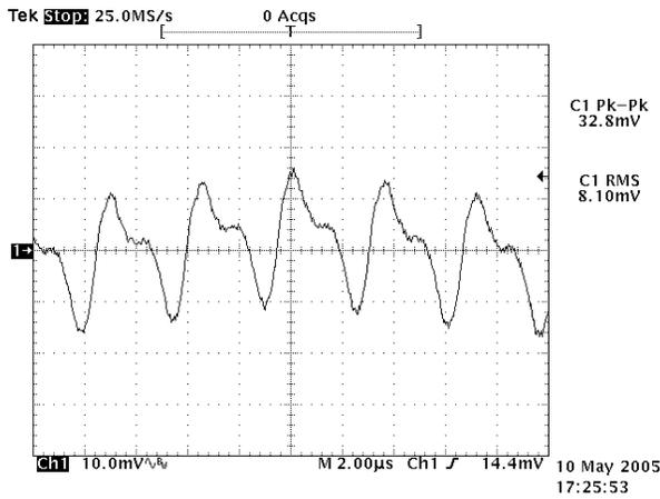
**Figure 3:** Output ripple & noise at 36Vin, 8.0V/3A out
