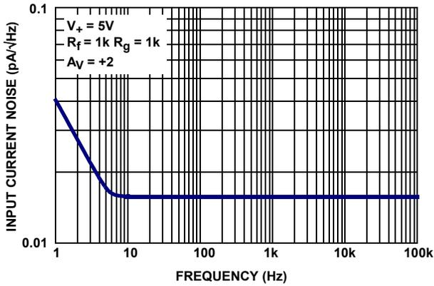
FIGURE 13. INPUT CURRENT NOISE DENSITY vs FREQUENCY
