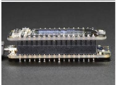
Finally, there's the "Stacking Header" option. This one is sort of the best-of-both-worlds. You get the ability to plug into a
