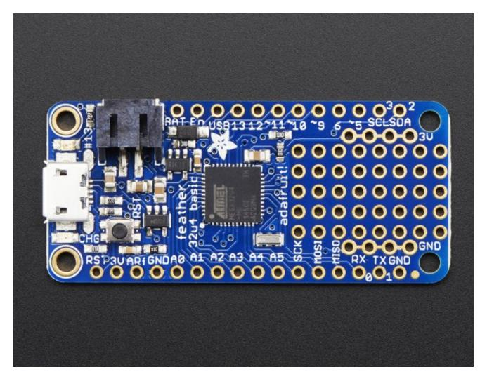
At the Feather 32u4's heart is at ATmega32u4 clocked at 8 MHz and at 3.3V logic, a chip setup we've had tons of experience with as <u>it's the same as the Flora (http://adafru.it/dVl)</u>. This chip has 32K of flash and 2K of RAM, with built in USB so not only does it have a USB-to-Serial program & debug capability built in with no need for an FTDI-like chip, it can also act like a mouse, keyboard, USB MIDI device, etc.
