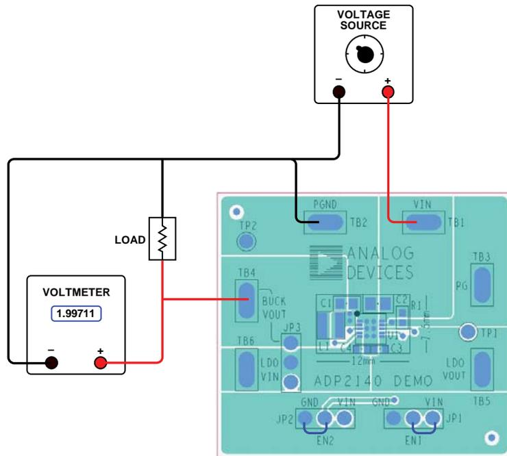
Figure 3. Buck Output Voltage Regulation Measurement Setup
