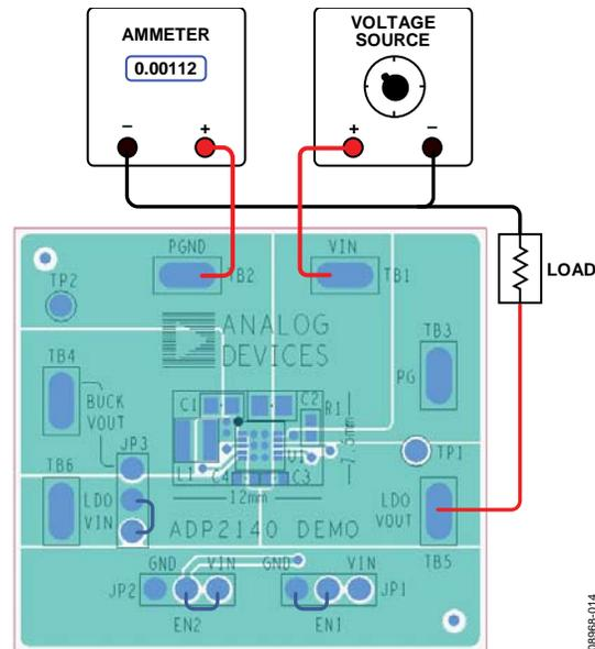
Figure 14. LDO Ground Current Measurement
