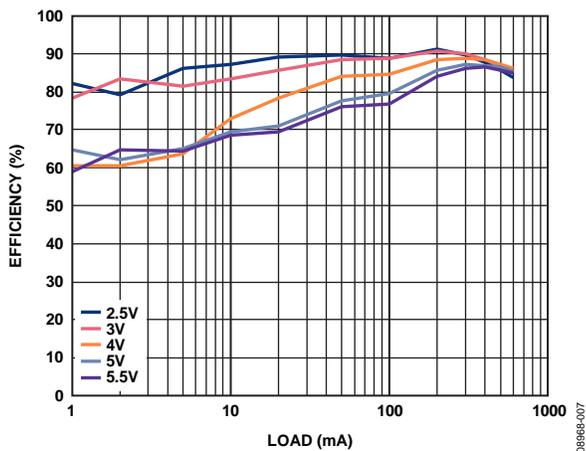
Figure 7. Efficiency vs. Input Voltage and Load
