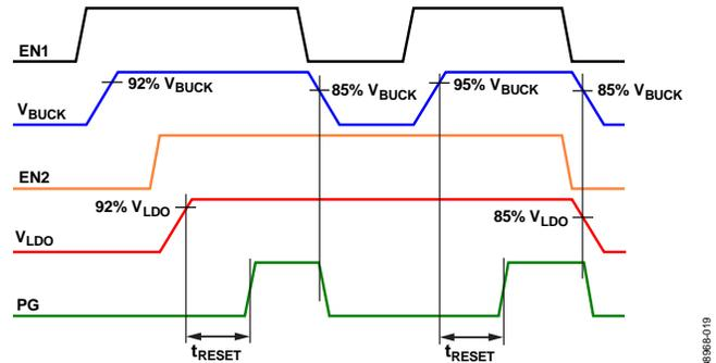
Figure 19. Individual Activation Mode, Both Regulators Sensed
