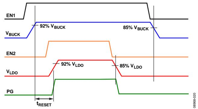
Figure 20. Individual Activation Mode, Only One Regulator (Buck) Sensed
