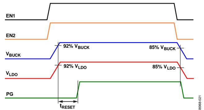
Figure 21. Individual Activation Mode, No Activation/Deactivation Delay Between Regulators, EN1 and EN2 Pins Tied Together
