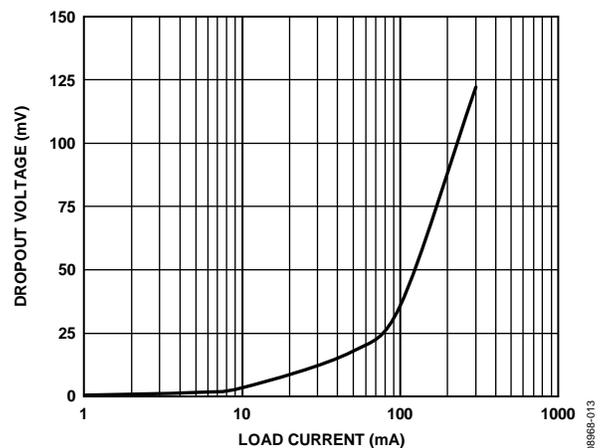
Figure 13. Dropout Voltage vs. Load Current
