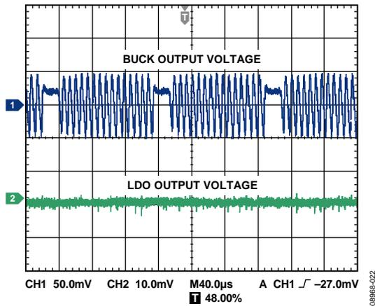
Figure 22. LDO as a Post Regulator,  $V_{OUT} = 1.8\text{ V}$ , Load Current = 50 mA,  $V_{OUT2} = 1.2\text{ V}$ , Load Current = 50 mA
