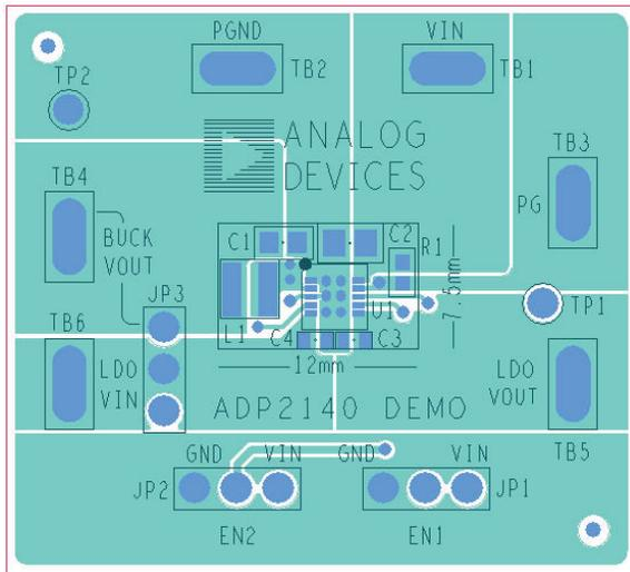
Figure 24. Typical Board Layout, Top Side
