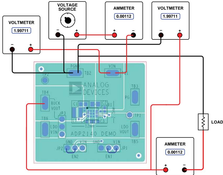
Figure 6. Buck Efficiency Measurement
