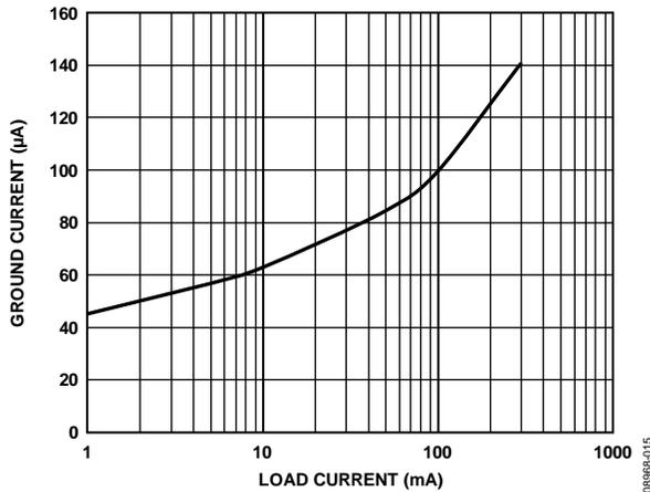
Figure 15. Ground Current vs. Load Current
