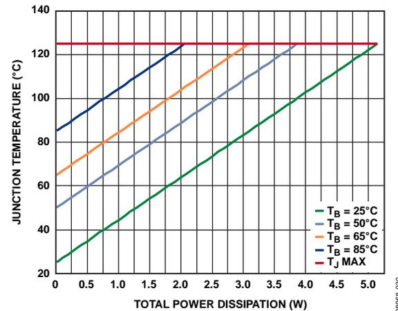
Figure 30.  $T_B = \text{Various Temperatures}$ , LFCSP
