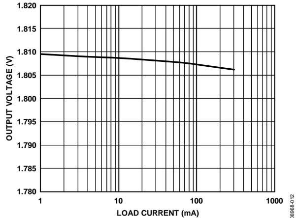
Figure 12. Output Voltage vs. Load Current
