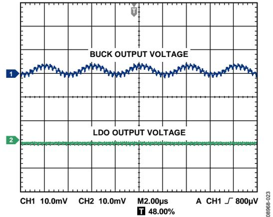
Figure 23. LDO as a Post Regulator,  $V_{OUT} = 1.8\text{ V}$ , Load Current = 500 mA,  $V_{OUT2} = 1.2\text{ V}$ , Load Current = 50 mA
