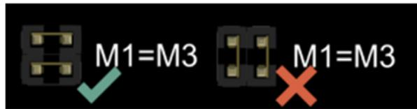
Correct and incorrect method of shorting the pins
