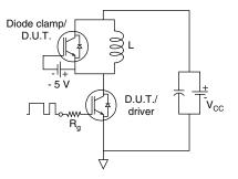
Fig. 14 - Switching Loss Test Circuit
