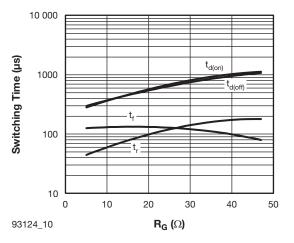
Fig. 10 - Typical IGBT Switching Time vs.  $R_g$   $T_J$  = 125 °C, L = 500  $\mu$ H, V<sub>CC</sub> = 600 V,  $R_g$  = 5  $\Omega,$  V<sub>GE</sub> = 15 V
