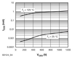
Fig. 4 - Typical IGBT Zero Gate Voltage Collector Current
