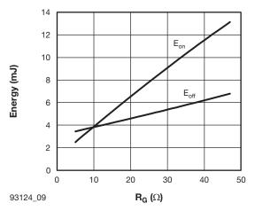
Fig. 9 - Typical IGBT Energy Loss vs.  $R_g$   $T_J$  = 125 °C,  $I_C$  = 75 A, L = 500  $\mu H,$   $V_{CC}$  = 600 V,  $V_{GE}$  = 15 V
