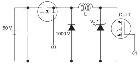
\* Driver same type as D.U.T.; V<sub>C</sub> = 80 % of V<sub>ce(max)</sub> \* Note: Due to the 50 V power supply, pulse width and inductor
