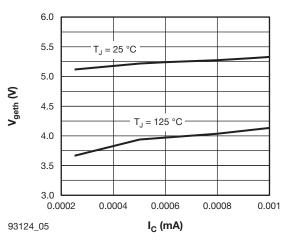
Fig. 5 - Typical IGBT Threshold Voltage
