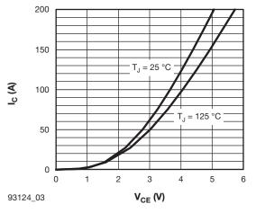
Fig. 3 - Typical IGBT Collector Current Characteristics
