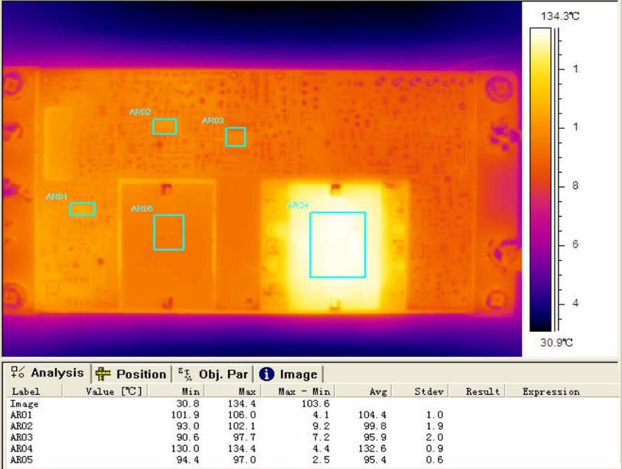
Figure 21 Thermal image, 48V<sub>in</sub>, 30V<sub>o</sub>, full load, room temperature
