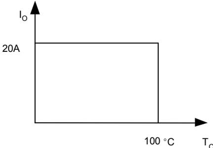
Figure 20 Output power derating curve, T<sub>c</sub>: temperature test point on baseplate, see Figure 19
