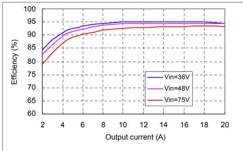
Figure 1 Efficiency vs. output current,  $T_a=25^{\circ}\text{C}$ ,  $T_c=40^{\circ}\text{C}$ ,  $V_o=30\text{V}$
