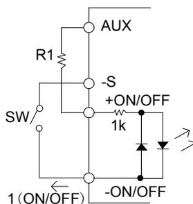
Figure 13 Connection of remote ON/OFF control (B)
