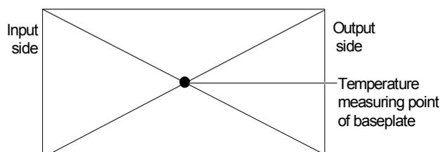
Figure 19 Temperature test point on base plate
