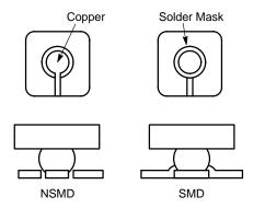
Figure 5. Solder Mask versus Non–Solder Mask Definition
