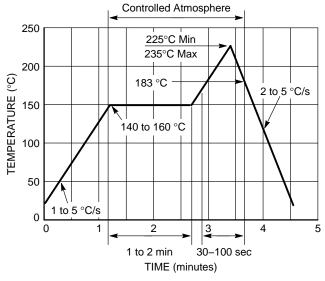
Figure 6. Solder Reflow Profile
