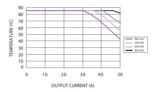
Figure 2 - Safe Operating Area Vin = 12 V, Output Voltage = 1.2 V (See Note A)
