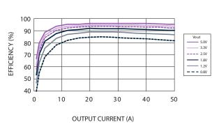
Figure 3 - Efficiency vs Load Current Vin = 12 V (See Note B)
