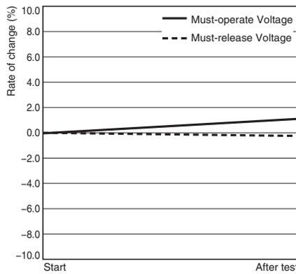
Characteristics were measured after applying vibration at a frequency of 5 to 200 to 5 Hz, acceleration of  $44.1 \text{ m/s}^2$  to the test piece (not energized) for 2 hours each in 3 directions. The percentage rate of change is the average value for all of the samples.
