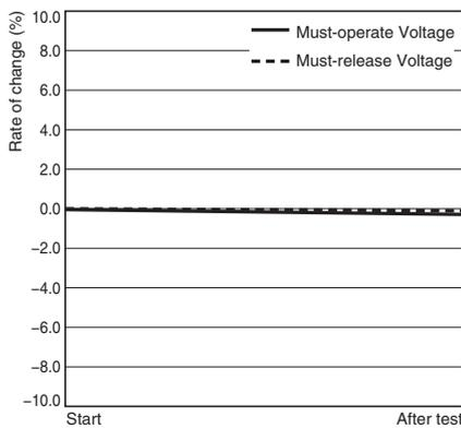
Characteristics were measured after applying a shock of  $490 \text{ m/s}^2$  to the test piece 3 times each in 6 directions along 3 axes. The percentage rate of change is the average value for all of the samples.
