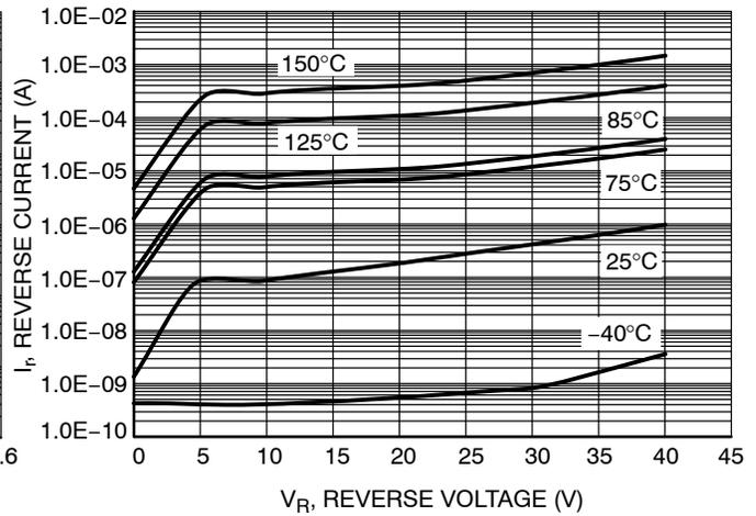
Figure 2. Leakage Current
