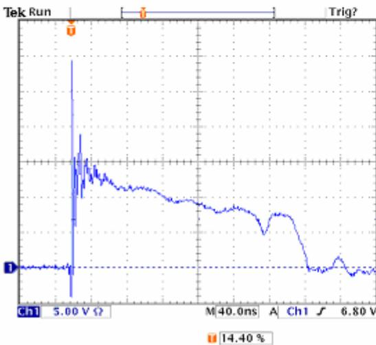
Figure 2 . Positive 8 kV Contact per IEC 6100-4-2
