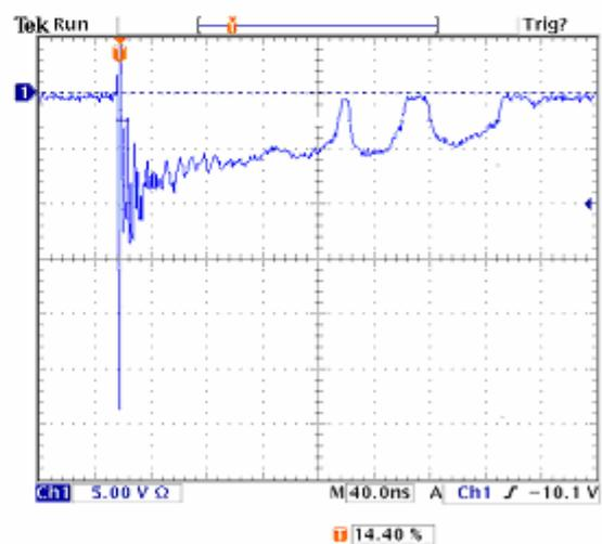
Figure 3. Negative 8 kV Contact per IEC 6100-4-2
