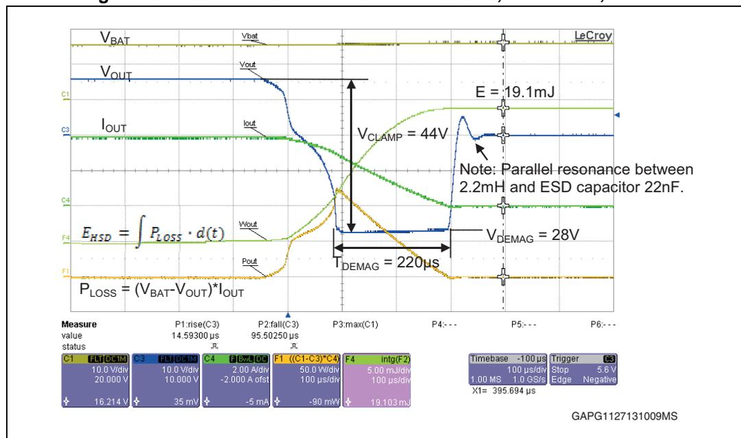
As seen from the oscillogram, measured values are close to the theoretical calculation:  $E_{\text{HSD}} = 19.1 \text{ mJ}$  (20.1 mJ calculated),  $T_{\text{DEMAG}} = 220 \mu\text{s}$  (235  $\mu\text{s}$  calculated).
