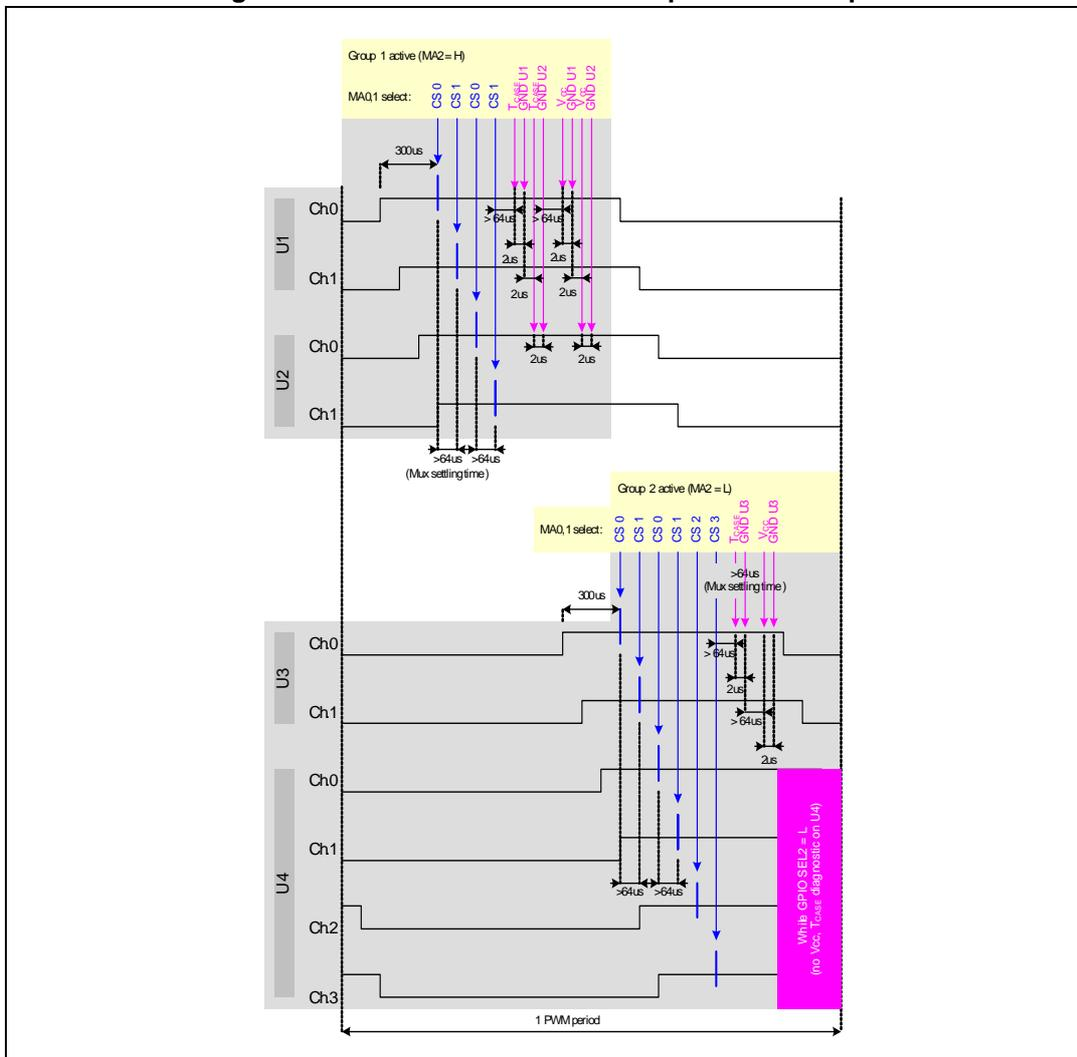
The best trigger position for the  $V_{CC}$ /Temp and the GND voltage measurement is usually after the rising edge of channel with highest phase shift, when all PWM channels are already activated. At that point the GND signal is stable (note that this statement is not valid during power limitation or thermal shutdown).
