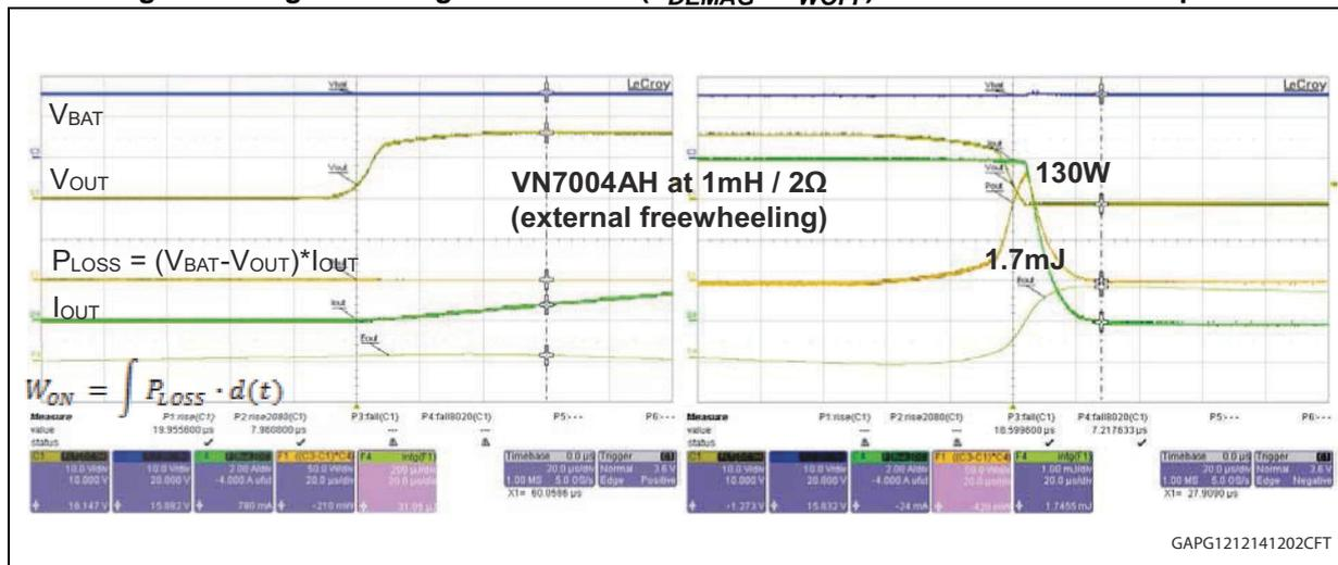
Measured losses (1 mH at 2 Ω):  $W_{ON} \sim 0.04 \text{ mJ}$ ,  $W_{OFF} \sim 1.75 \text{ mJ}$
