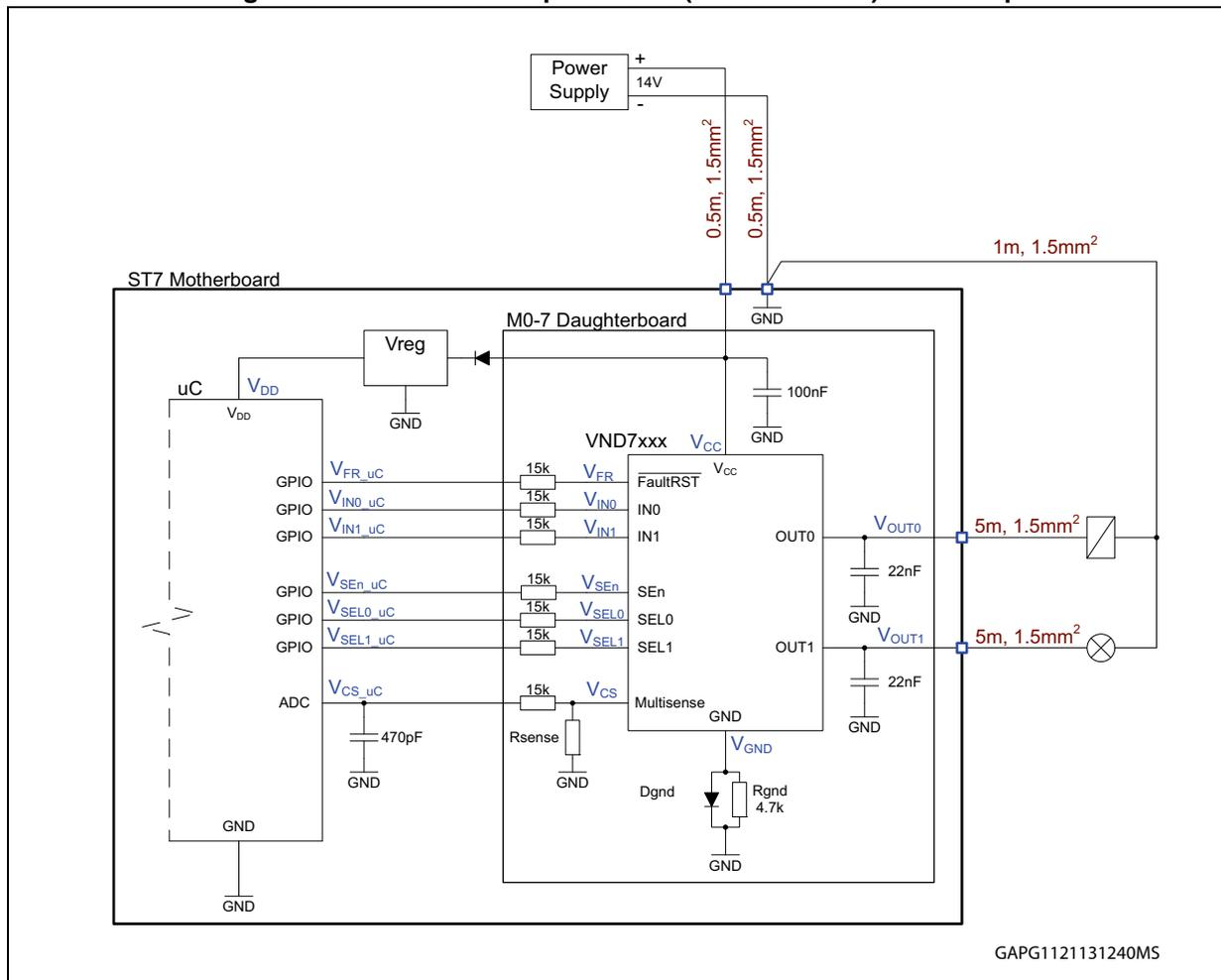
Figure 6. Measurement example ( $t_{\text{DEMAG}} > t_{\text{D\_STBY}}$ ) without GND resistor
