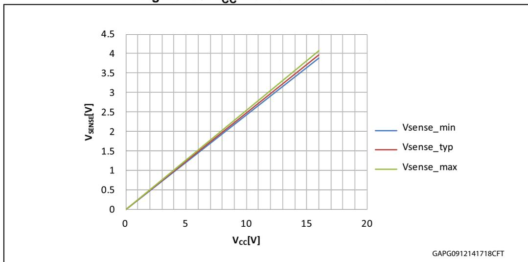
Applying limit cases of transfer coefficients show possible inaccuracy of V<sub>CC</sub> monitoring.
