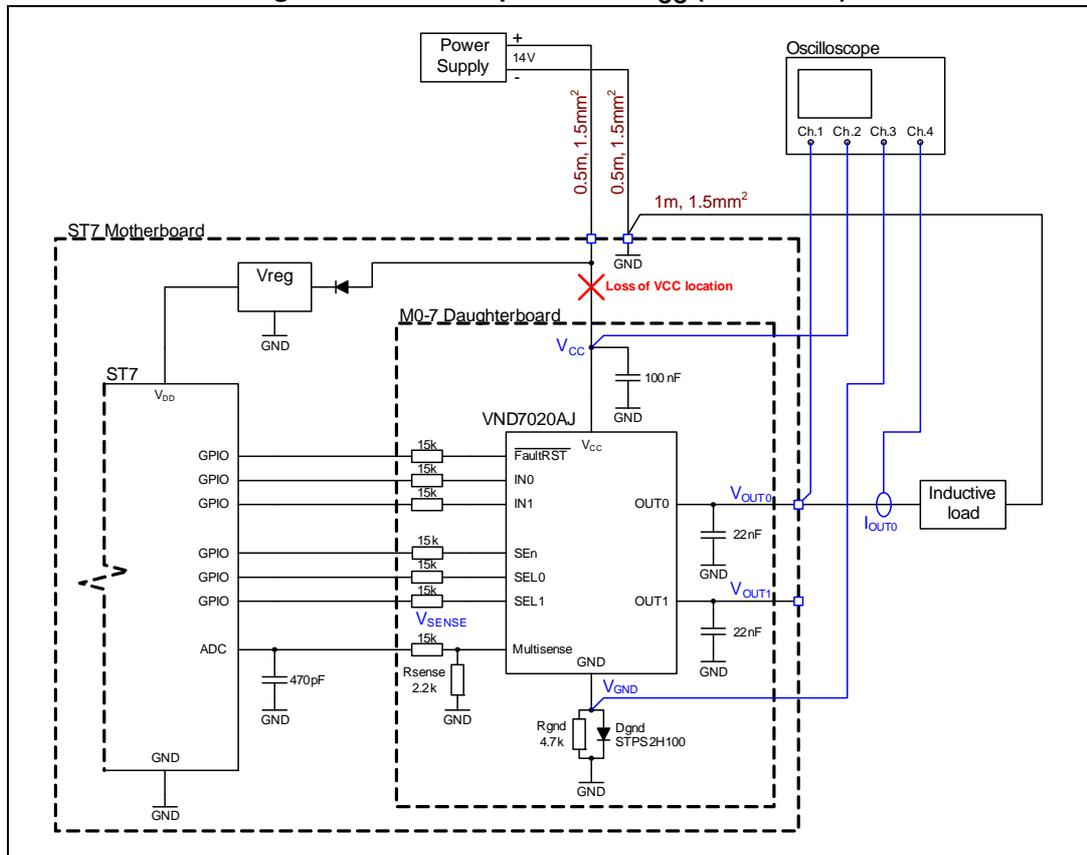
Figure 85. Loss of  $V_{CC}$  (VND7020AJ, 1 mH/ 3.5  $\Omega$ , 100 nF)
