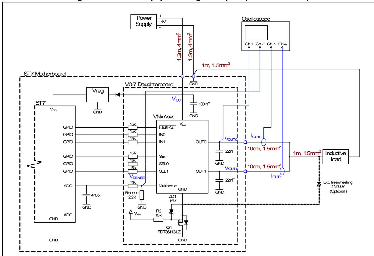
Figure 142. Bulb with 10 μH (VND7040AJ, Ch.0 + Ch.1)
