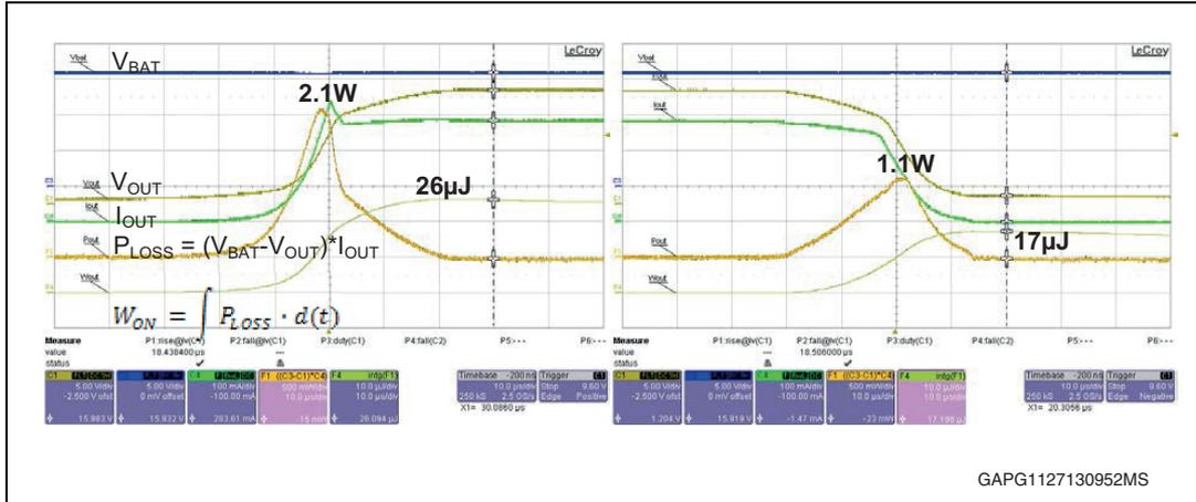
Measured losses:  $W_{ON} \sim 26 \mu J$ ,  $W_{OFF} \sim 17 \mu J$
