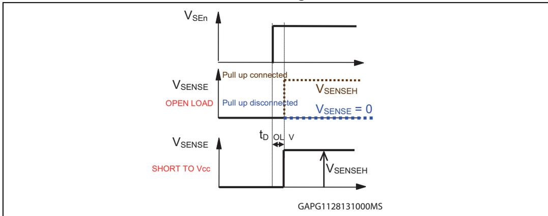
Table 26. MultiSense pin levels in off-state
