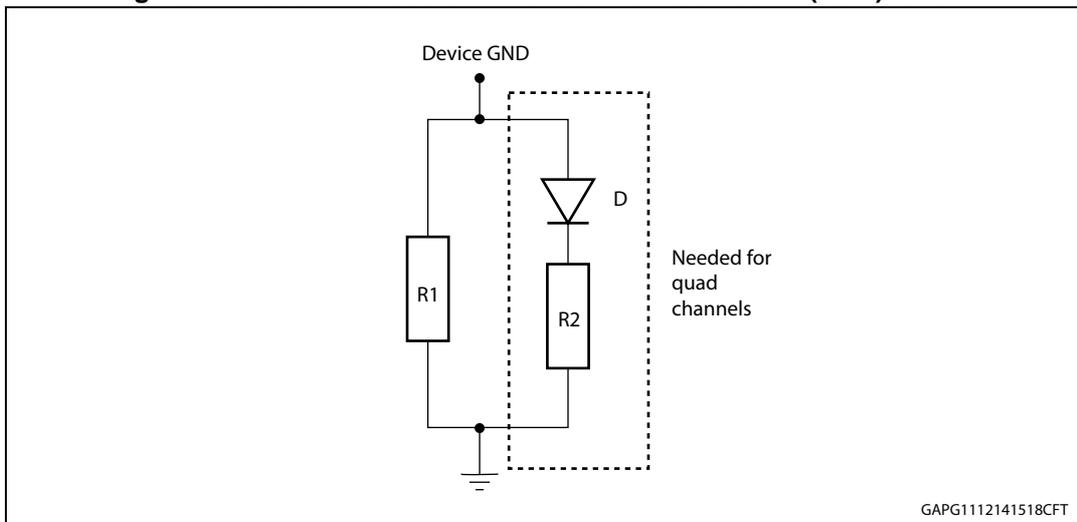
A second solution with an additional branch in parallel (R2 + low drop diode D) depends on specific considerations. The Table 8 gives a suggestion according to the Hybrid device type and to the logic level of Input pin adopted.
