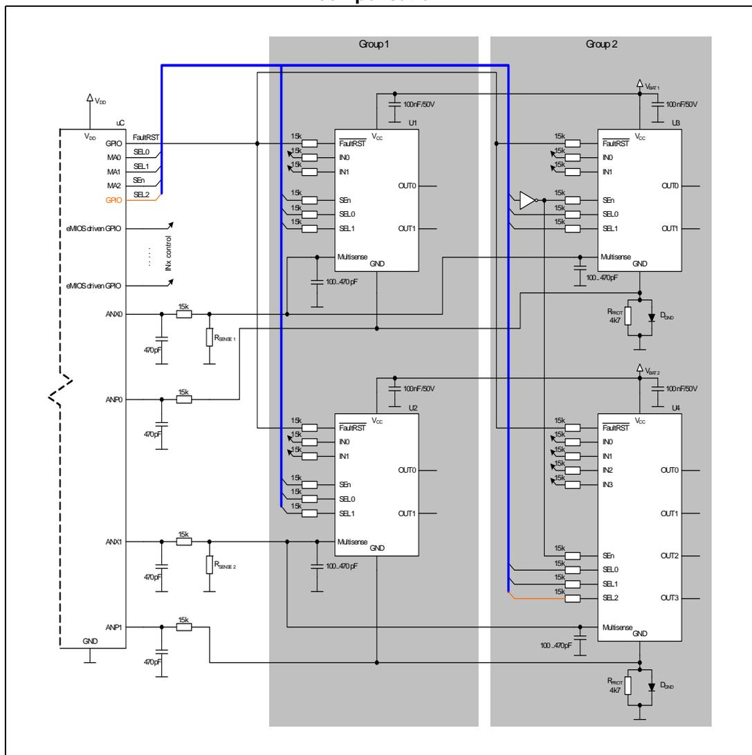
To eliminate the effect of the GND shift variation, it is important to measure the GND voltage and  $V_{CC}$  / Temp signal in the same time (ideally) or with a few  $\mu\text{s}$  delay. Possible solutions are shown in the [Figure 122](#).
