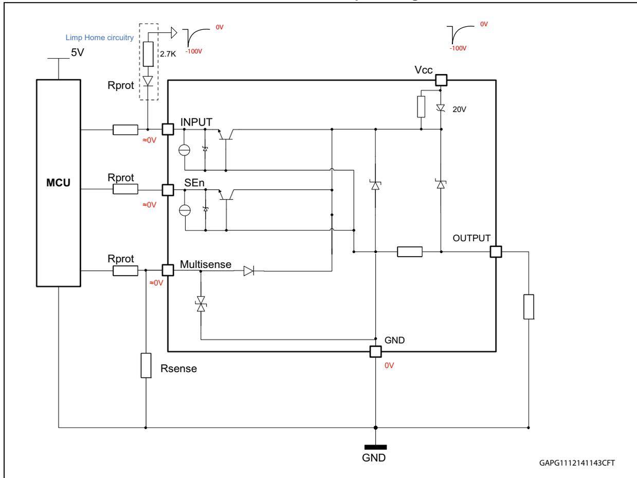
Anyway, to be compliant with the ISO 7637-2 (edition 2011) test pulse 1 level IV and 2a level IV, it is recommended to adopt a GND network in order to limit the current flowing through the internal clamp structure.
