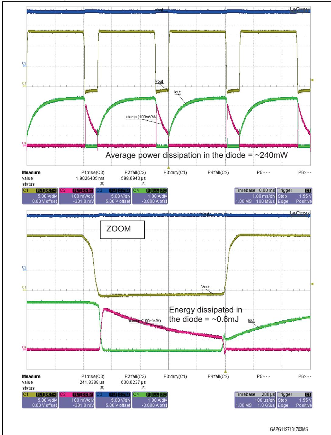
Negative ISO pulse exposure on V<sub>CC</sub> line:
