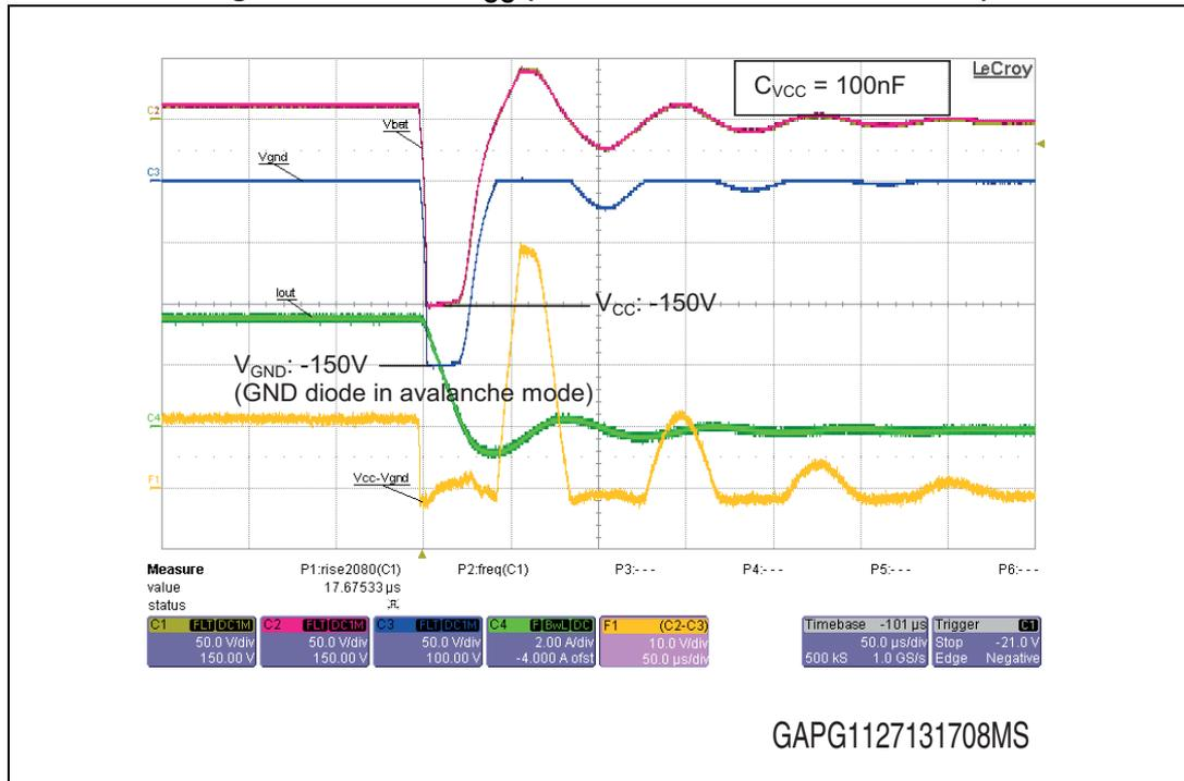
Most of the demagnetization energy (Figure 85) is absorbed by the GND network diode (in avalanche mode). The voltage peak on the  $V_{CC}$  and GND pin is  $\sim$ -150 V (equal to break down voltage of the diode). The device channel stays on for whole demagnetization phase  $\sim$ 30  $\mu$ s. A positive overshoot on  $V_{CC}$  is seen at the end of demagnetization phase, due to the resonance between the  $V_{CC}$  capacitor and load inductance.
