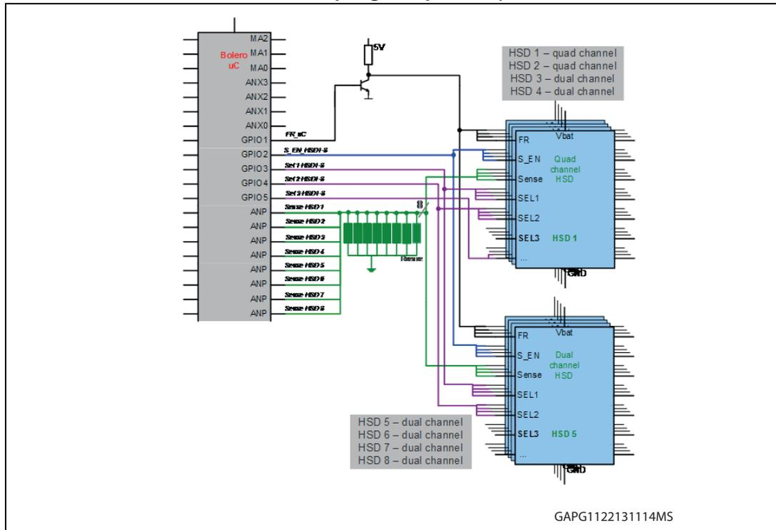
Figure 33. FaultRST pin handling concept
