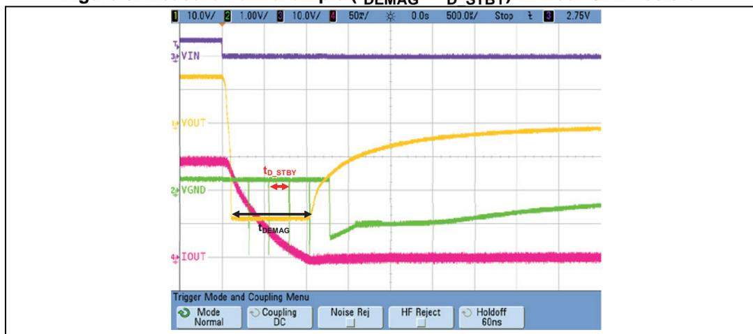
Figure 7. Measurement example ( $t_{DEMAG} > t_{D\_STBY}$ ) with 4.7 kΩ GND resistor
