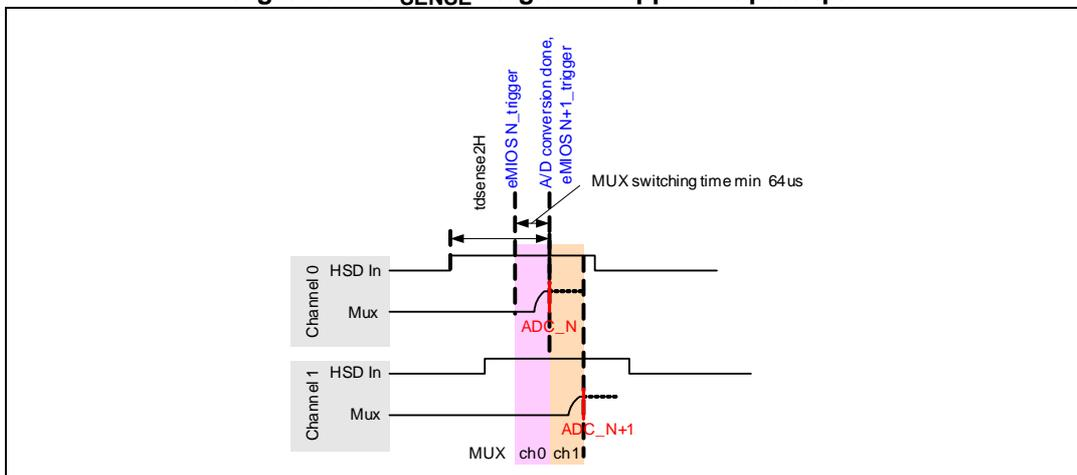
Example configuration applying 0 % CPU load (MUX switching done by microcontroller HW peripherals)
