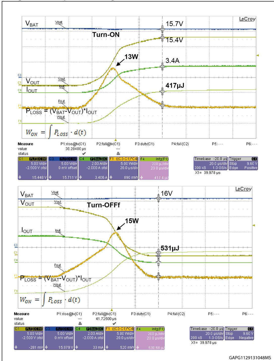
As seen from the measurement, in this case the switching shapes are not absolutely symmetrical so the turn-off loss is slightly higher (531 µJ turn-off versus 417 µJ turn-on). Measured values are slightly below the calculated value (569 µJ).
