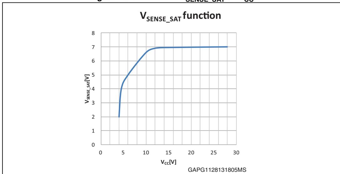
Figure 93. Behavior of  $I_{SENSE\_SAT}$  vs  $V_{CC}$
