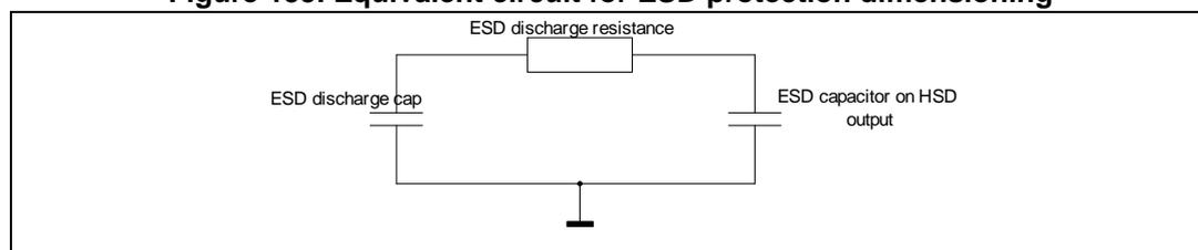
A preliminary estimation of the capacitor value can be obtained applying the following formula:
