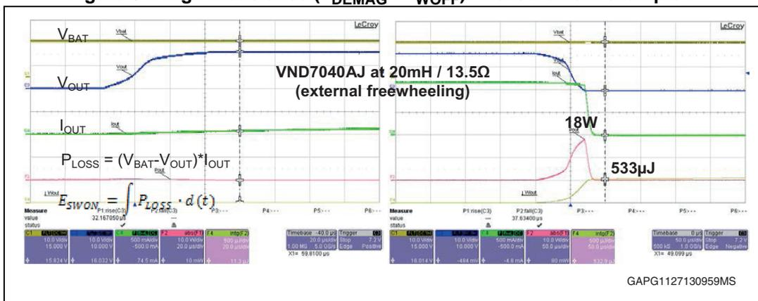
Measured losses (20 mH at 13.5 Ω):  $W_{ON} \sim 11 \mu\text{J}$ ,  $W_{OFF} \sim 533 \mu\text{J}$
