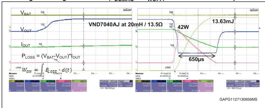
Measured T<sub>DEMAG</sub>: 6500 µs (633 µs calculated)
