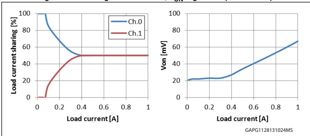
Figure 139. Current sense behavior at low current (VND7140AJ)
