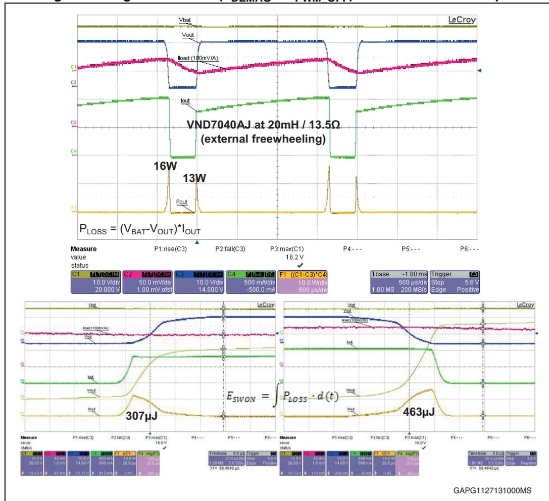
Measured losses (20 mH at 13.5  $\Omega$ ):  $W_{ON} \sim 307 \mu J$  ( $I_{OUT} \sim 1 A$ )
