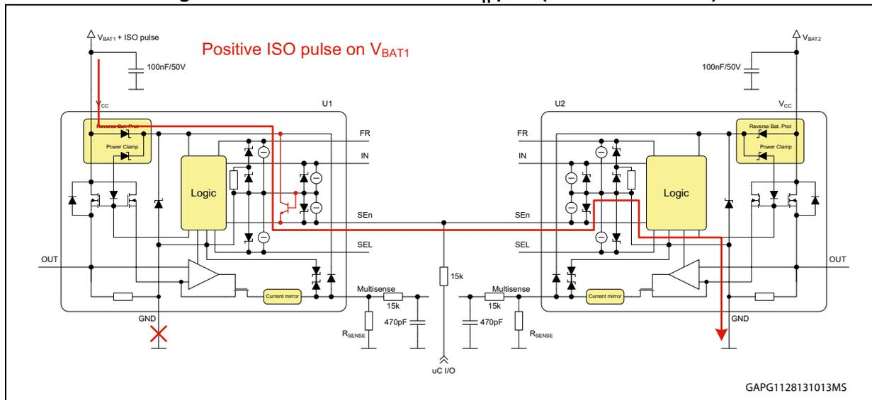
Direct connection of SE<sub>n</sub> pins is not safe in the following cases:
