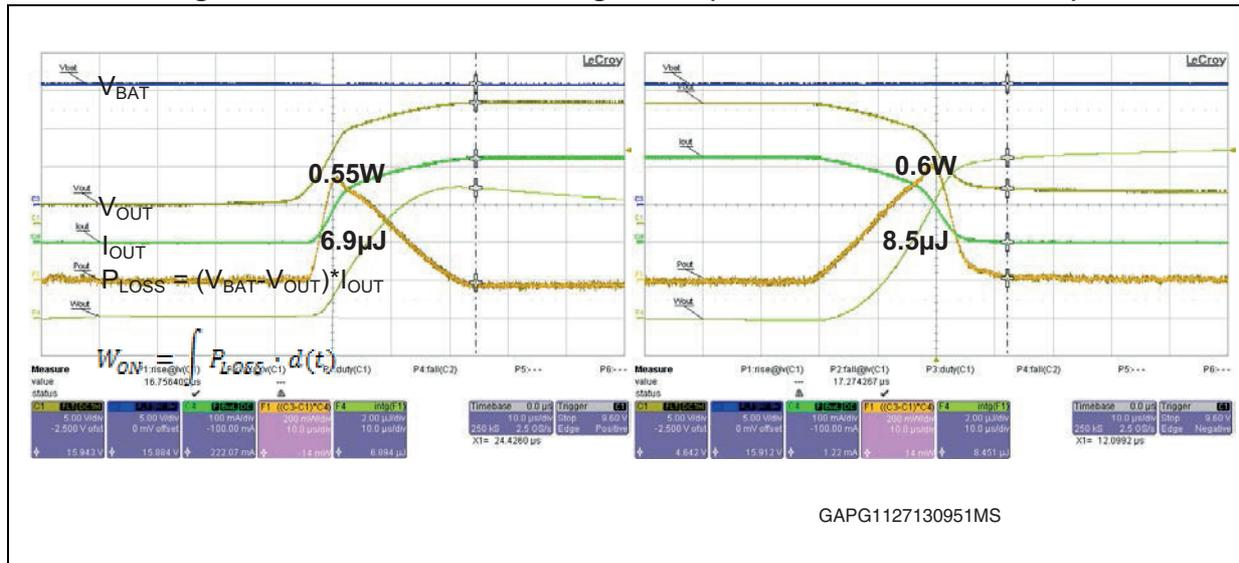
Measured losses:  $W_{ON} \sim 6.9 \mu\text{J}$ ,  $W_{OFF} \sim 8.5 \mu\text{J}$
