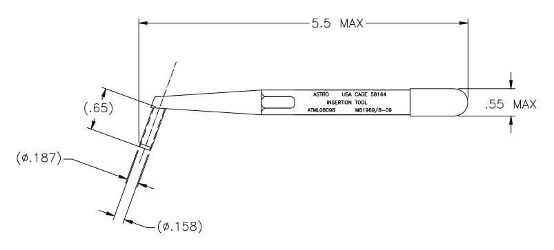
3. WITH TIPS CLOSED AROUND A .1570 +.0000/-.0002 DIA PIN, MAX GAP TO BE .006.
