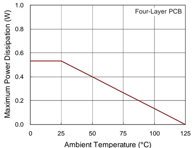
Figure 4. Derating Curve of Maximum Power Dissipation
