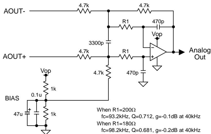
Figure 11. External 2<sup>nd</sup> order LPF Circuit Example (using op-amp with single power supply)
