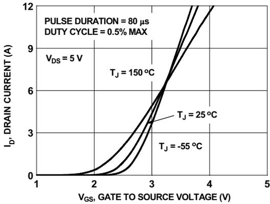
**Figure 5. Transfer Characteristics**
