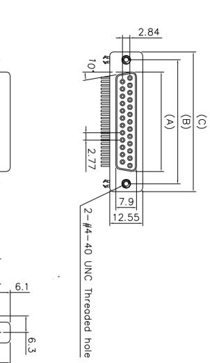
Insulator Resistance: 1000M ohms min. at DC 500V Contact Resistance: 30m ohms max. at DC 100mA
