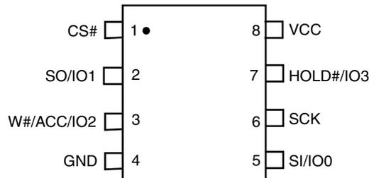
**Figure 3. 8-contact USON (5 x 6 mm) Package**
