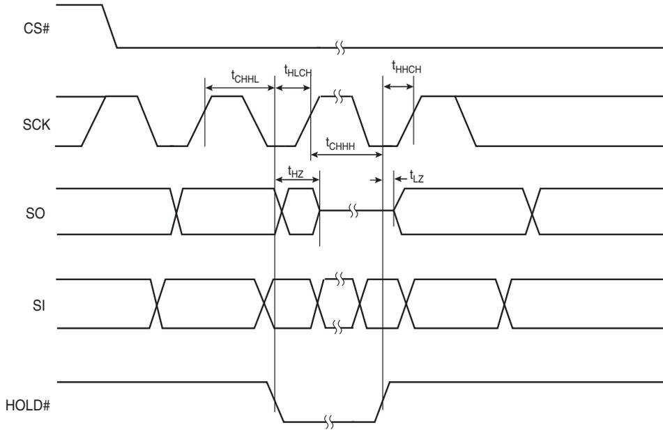
**Figure 48. Write Protect Setup and Hold Timing during WRR when SRWD = 1**
