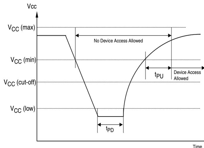
**Table 19. Power-Up / Power-Down Voltage and Timing**
