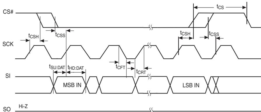
Figure 46. SPI Mode 0 (0,0) Output Timing
