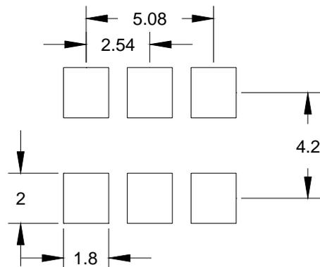
Note: XPRESSO LVDS XO's are designed to fit on Industry standard, 6 pad, layouts.
