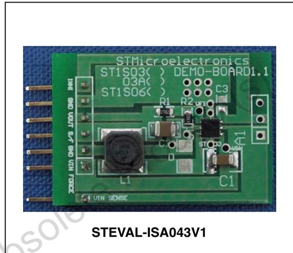
capacitors results in a low, predictable output ripple. To clamp the error amplifier reference voltage, this device includes a soft-start control block generating a voltage ramp.
