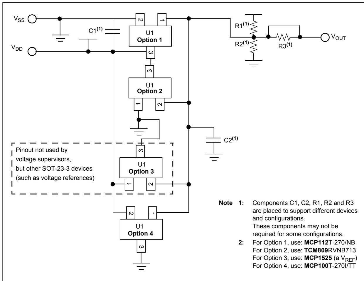
**TABLE 2-1: VOLTAGE SUPERVISOR / VOLTAGE DETECTOR DEVICES AND EVAL BOARD CIRCUIT/FOOTPRINT OPTION**
