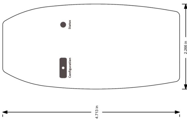
Figure 2. Mechanical drawing for WzzardC™ Commercial models
