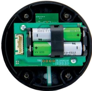
In most installations you will only need to place the batteries in the battery holder. But in high vibration environments you should also use the optional battery retaining clip. Do not use excessive force while placing or removing the clip, as you can break it.
