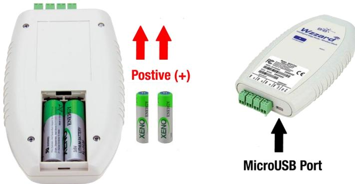
Remove back cover. Insert both batteries with the positive (+) towards the terminal blocks.
