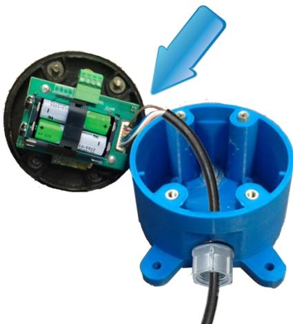
Connect your sensor to the wires running from the node's conduit. Consult the charts below for wire colors and connections.
