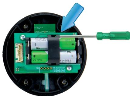
As with all batteries, these are a fire, explosion, and severe burn hazard. Do not burn or expose them to high temperatures. Do not recharge, crush, disassemble, or expose the contents to water. Properly dispose of used batteries according to local regulations by taking it to a hazardous waste collection site, an e-waste disposal center, or other facility qualified to accept lithium batteries.
