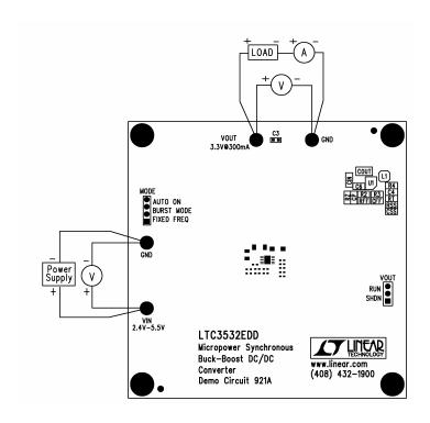
Figure 1. Proper Measurement Equipment Setup
