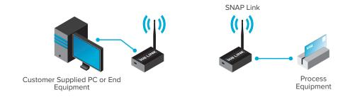
One SNAP Link Adaptor controls multiple SNAP Link serial wireless adapters (either RS-232 or RS-485/422).
