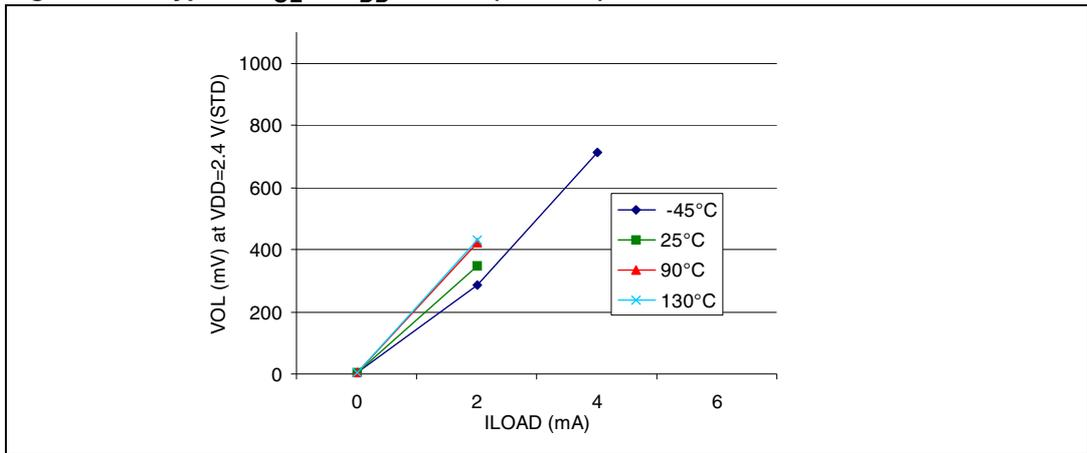
Figure 100. Typical  $V_{OL}$  at  $V_{DD} = 3\text{ V}$  (std I/Os)
