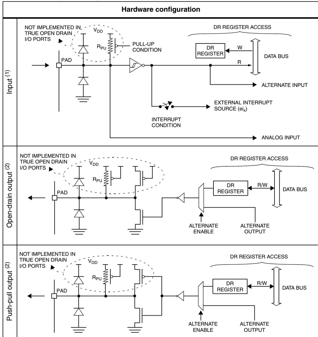
1. When the I/O port is in input configuration and the associated alternate function is enabled as an output, reading the DR register will read the alternate function output status.
