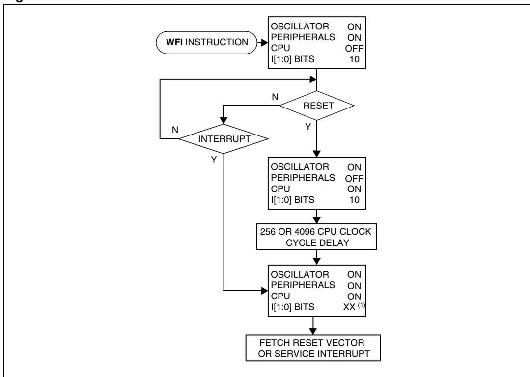
Note: Before servicing an interrupt, the CC register is pushed on the stack. The I[1:0] bits of the CC register are set to the current software priority level of the interrupt routine and recovered when the CC register is popped.
