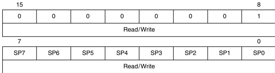
The Stack pointer is a 16-bit register which is always pointing to the next free location in the stack. It is then decremented after data has been pushed onto the stack and incremented before data is popped from the stack (see [Figure 12](#)).
