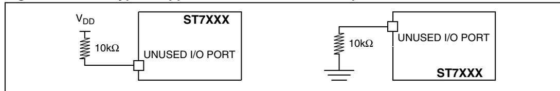
1. I/O can be left unconnected if it is configured as output (0 or 1) by the software. This has the advantage of greater EMC robustness and lower cost.
