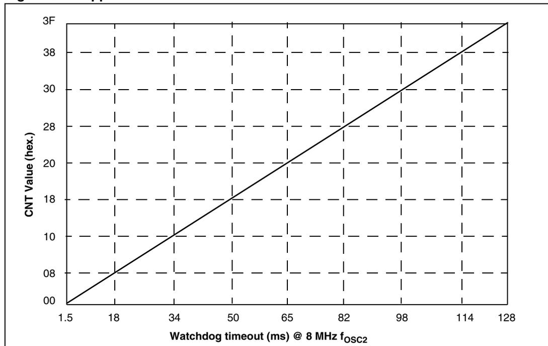
**Figure 39. Exact timeout duration ( $t_{min}$  and  $t_{max}$ )**
