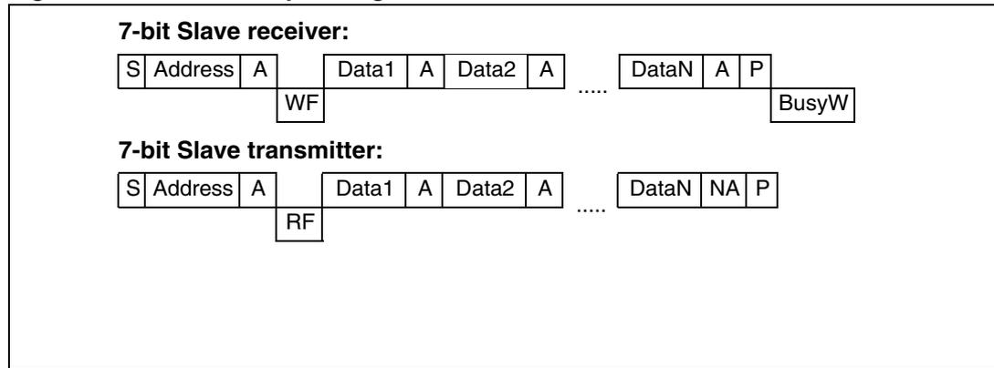
Legend: S = Start, P = Stop, A = Acknowledge, NA = Non-acknowledge, WF = WF event, WFx bit is set (with interrupt if ITWEx=1, after Stop or Restart conditions), cleared by reading the I2C3SSR register while no communication is ongoing.
