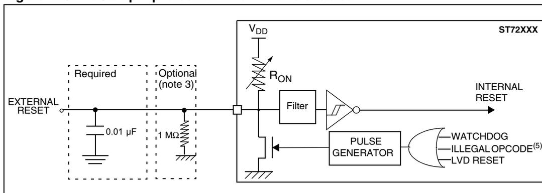
1. The reset network protects the device against parasitic resets.
