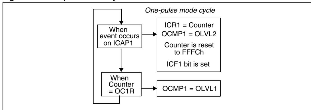
When a valid event occurs on the ICAP1 pin, the counter value is loaded in the ICR1 register. The counter is then initialized to FFFCh, the OLVL2 bit is output on the OCMP1 pin and the ICF1 bit is set.
