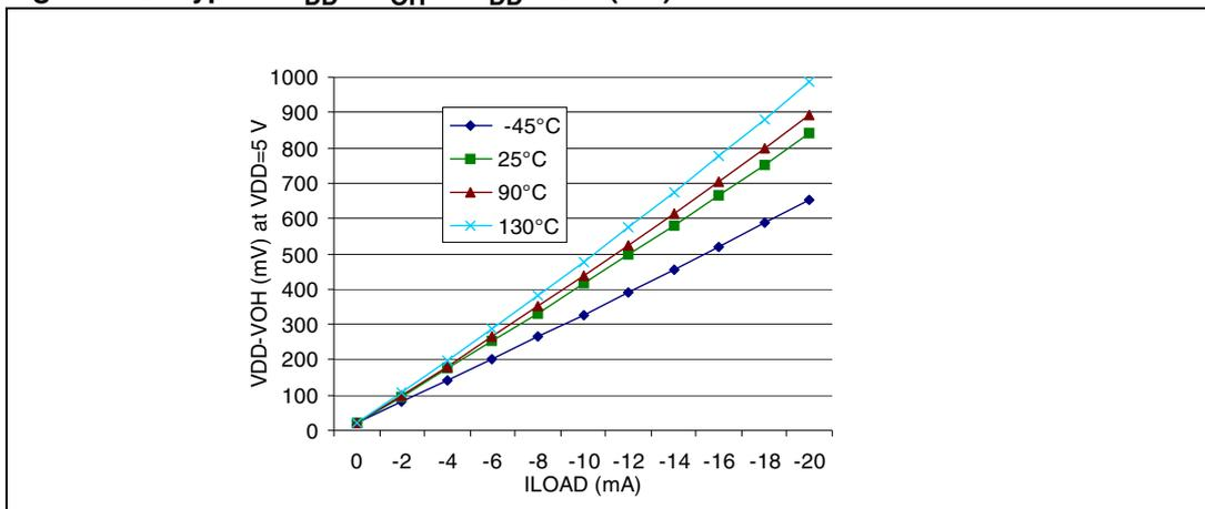
Figure 114. Typical  $V_{DD} - V_{OH}$  vs.  $V_{DD}$  (high sink)
