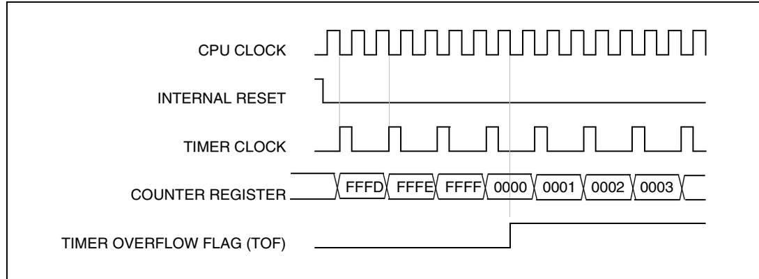
**Figure 45. Counter timing diagram, internal clock divided by 4**
