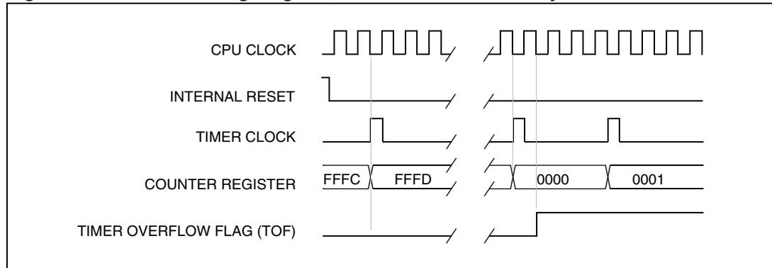
**Figure 46. Counter timing diagram, internal clock divided by 8**
