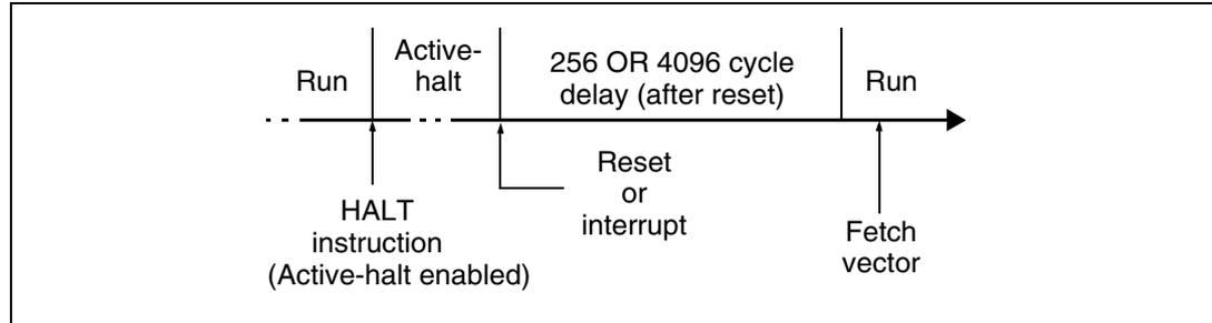
Figure 31. Active-halt mode flowchart
