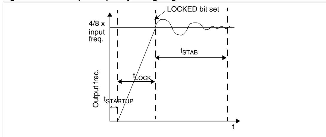
When the PLL is started, after reset or wakeup from Halt mode or AWUFH mode, it outputs the clock after a delay of  $t_{STARTUP}$
