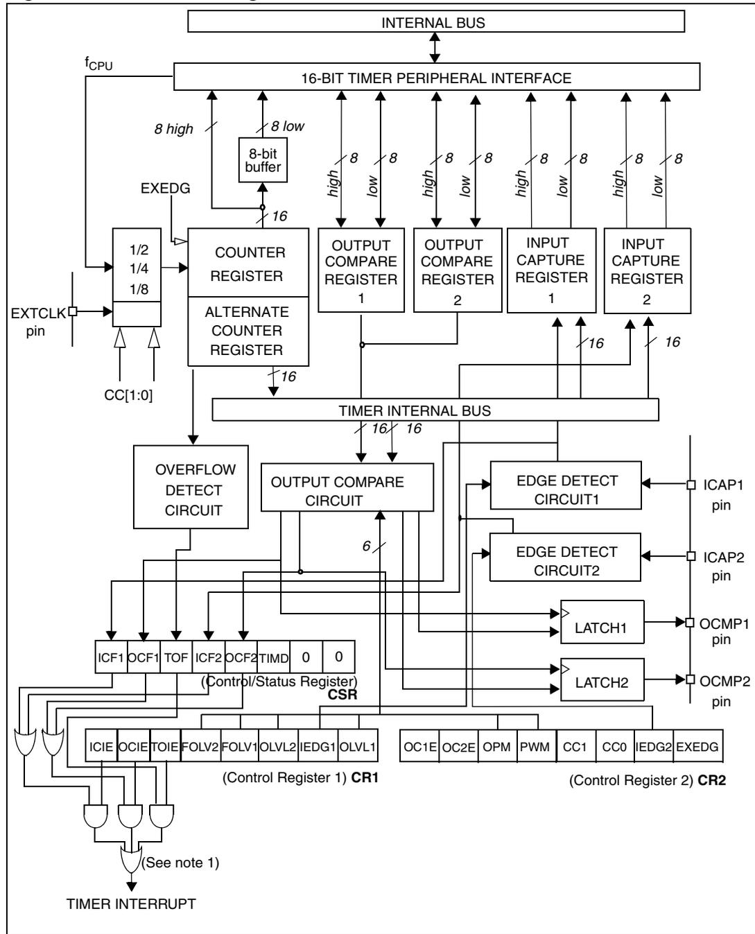
1. If IC, OC and TO interrupt requests have separate vectors, then the last OR is not present (See Device Interrupt Vector Table).
