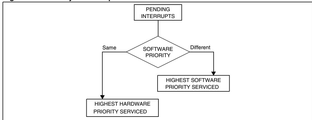
When an interrupt request is not serviced immediately, it is latched and then processed when its software priority combined with the hardware priority becomes the highest one.
