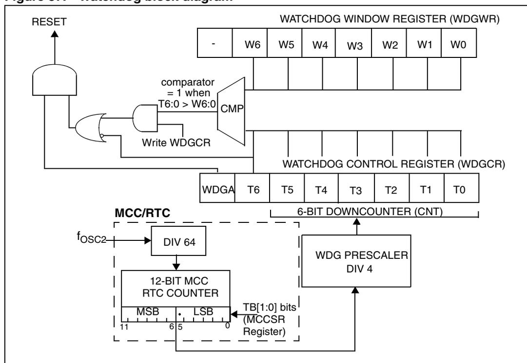
The application program must write in the WDGCR register at regular intervals during normal operation to prevent an MCU reset. This operation must occur only when the counter value is lower than the window register value. The value to be stored in the WDGCR register must be between FFh and C0h (see [Figure 38: Approximate timeout duration](#)):
