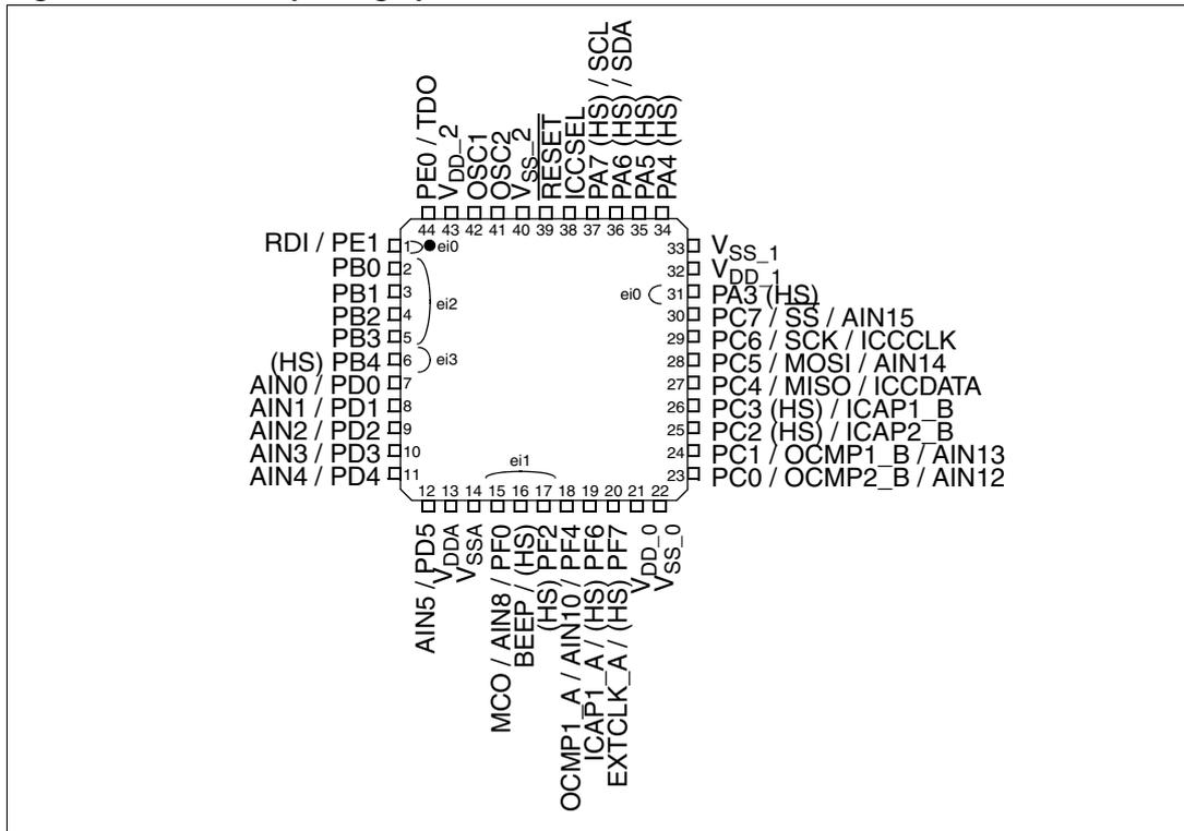
Figure 4. LQFP48 package pinout
