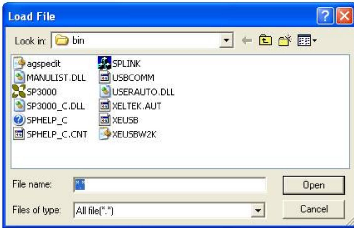
To select a data file to be loaded, the path and the file name should be entered into the name field. If the full path or the exact name of the file is unknown, then a partial path may be entered using wild cards, e.g. '\*.\*' or '\*.bin'.
