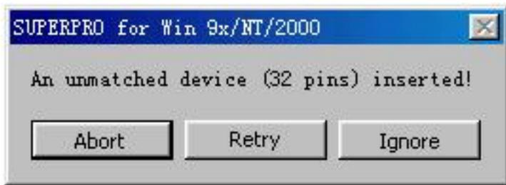
If Insertion Test finds errors, users can click Abort to stop the programming, or click Retry to run Insertion Test again, or click Ignore to program despite the errors.
