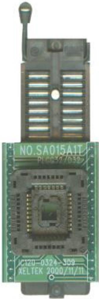
Note: usually the front side of the chip is placed upwards; but for PLCC 20-pin chip, it needs to be placed with the front side downwards. This method is called Dead Bug.
