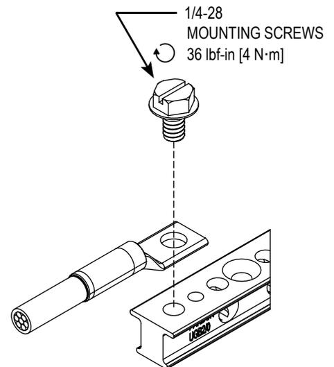
\* "MAIN" EQUIPMENT GROUNDING CONDUCTOR MAXIMUM OF 2/0 AWG COPPER CONDUCTOR
