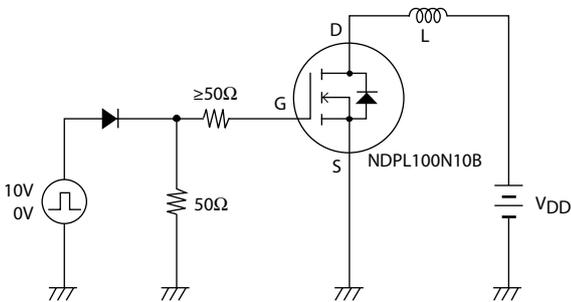
**Fig.2 Switching Time Test Circuit**
