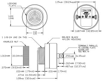
NOTE A: TERMINALS-.032 BRASS TIN PLATED, TAPPED FOR #6-32 SCREW. TWD #6-32 NICKEL PLATED BRASS SCREWS INCLUDED. WILL ACCEPT 1/4\* QUICK CONNECT. B: MOUNTING- REMOVE BLACK PLASTIC NUT AND INSERT THREADED FRONT THROUGH 1.25' HOLE PUNCHED IN PANEL, IF ORIENTATION IS NEEDED, NOTE LOCKING FLATS ON DRAWING SCREW NUT BACK ON. DO NOT OVERTIGHTEN.
