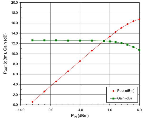
**P<sub>OUT</sub>/Gain versus P<sub>IN</sub> at 14 GHz**
