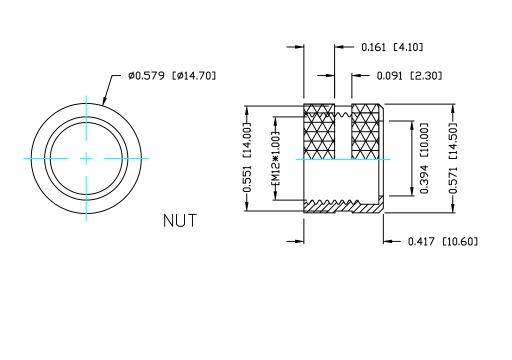
M12 FEMALE - CABLE MOUNT - SOLDER CUP - 3 POS.
