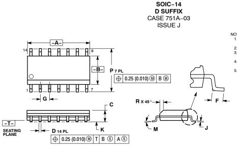
NOTES: 1. DIMENSIONING AND TOLERANCING PER ANSI Y14.5M, 1982. 2. CONTROLLING DIMENSION: MILLIMETER. 3. DIMENSIONS A AND B DO NOT INCLUDE MOLD PROTRUSION. 4. MAXIMUM MOLD PROTRUSION 0.15 (0.006) PER SIDE. 5. DIMENSION D DOES NOT INCLUDE DAMBAR PROTRUSION. ALLOWABLE DAMBAR PROTRUSION. SHALL BE 0.127 (0.005) TOTAL IN EXCESS OF THE D DIMENSION AT MAXIMUM MATERIAL CONDITION.
