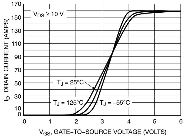
Figure 2. Transfer Characteristics
