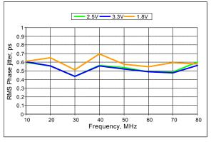
Figure 11. RMS Phase Jitter vs Frequency
