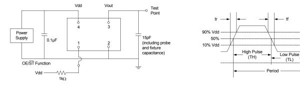
Figure 2. Test Circuit
