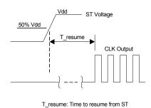
Figure 5. Standby Resume Timing (ST Mode Only)
