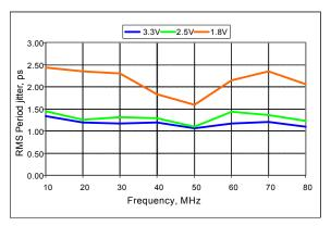
Figure 9. RMS Period Jitter vs Frequency
