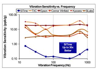
Figure 5. Vibration Robustness<sup>[5]</sup>
