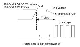
Figure 4. Startup Timing (OE/ST Mode)
