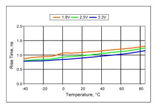
Figure 13. Rise Time vs Temperature, 75 MHz Output
