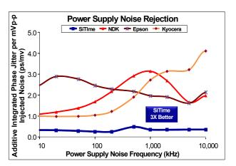
Figure 4. Power Supply Noise Rejection<sup>[4]</sup>
