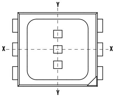
**Figure 14 Recommended Soldering Land Pattern**
