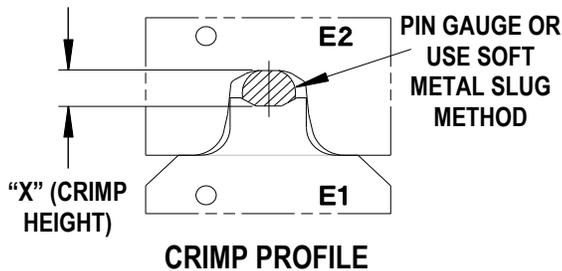
Use gauge pins or soft metal slug (solder) method to measure the “X” dimension. Verify tooling crimp height calibration by referring to the Go/No Go dimensions shown in the chart below.
