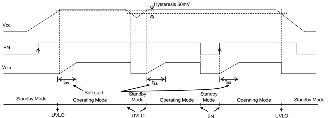
Figure 26. Soft-Start, Shutdown, UVLO Timing Chart
