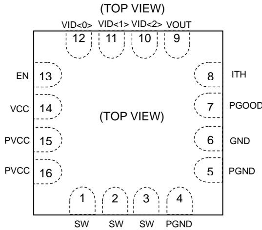
Figure 2. Pin Configuration
