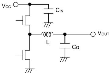
Figure 36. Input Capacitor
