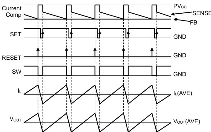
Figure 23. PWM Switching Timing Chart
