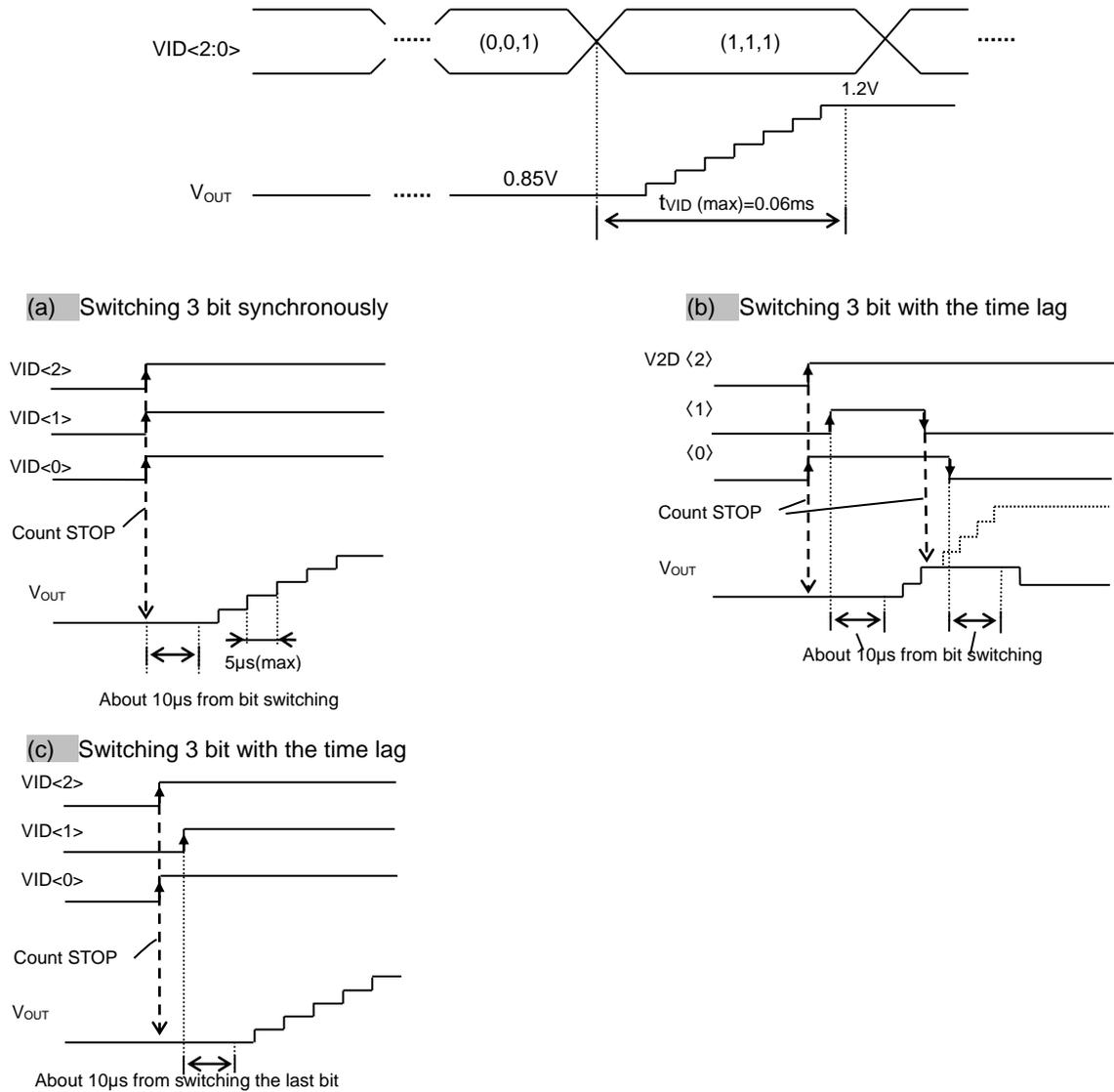
Figure 28. Timing Chart of Setting the Output voltage
