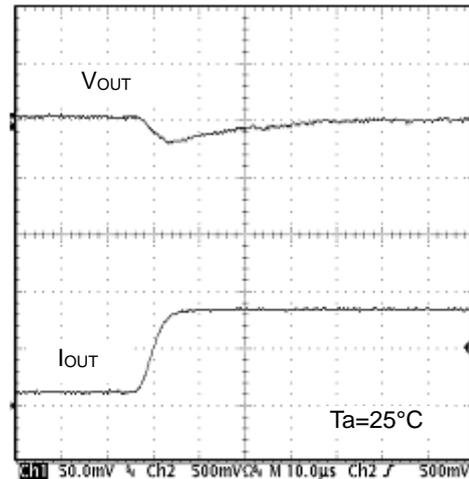
Figure 17. Transient Response (IO=125mA to 850mA, 2µA)
