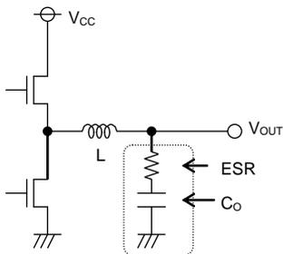
Figure 35. Output Capacitor
