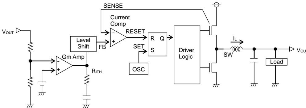
Figure 22. Diagram of Current Mode PWM Control
