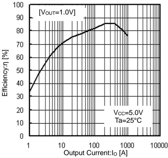
Figure 8. Efficiency vs Output
