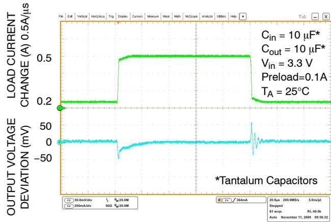
Figure 31. Load Transient Response –  $V_{out} = 5.0 V$
