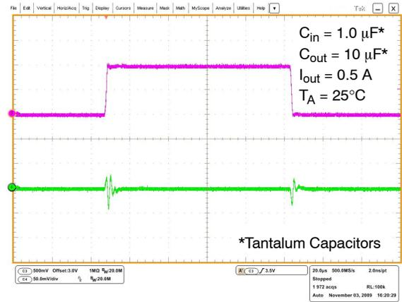
Figure 19. Line Transient Response –  $V_{out} = 1.5 V$
