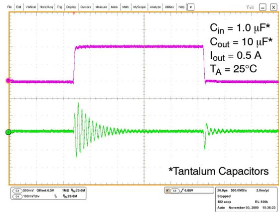
Figure 27. Line Transient Response –  $V_{out} = 5.0 V$
