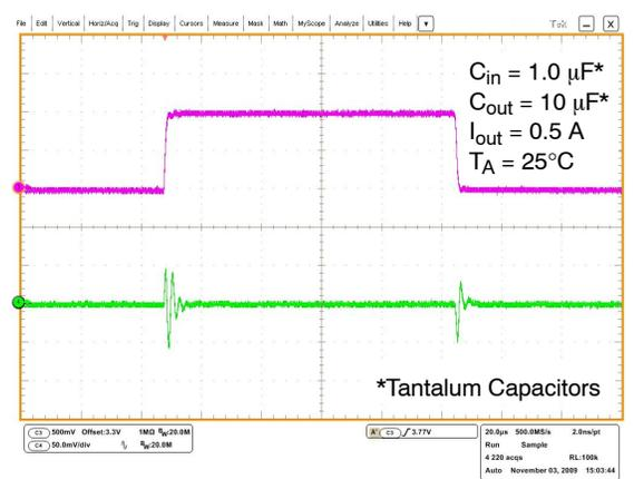
Figure 21. Line Transient Response –  $V_{out} = 1.8 V$
