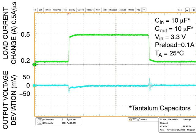
Figure 30. Load Transient Response –  $V_{out} = 3.3 V$
