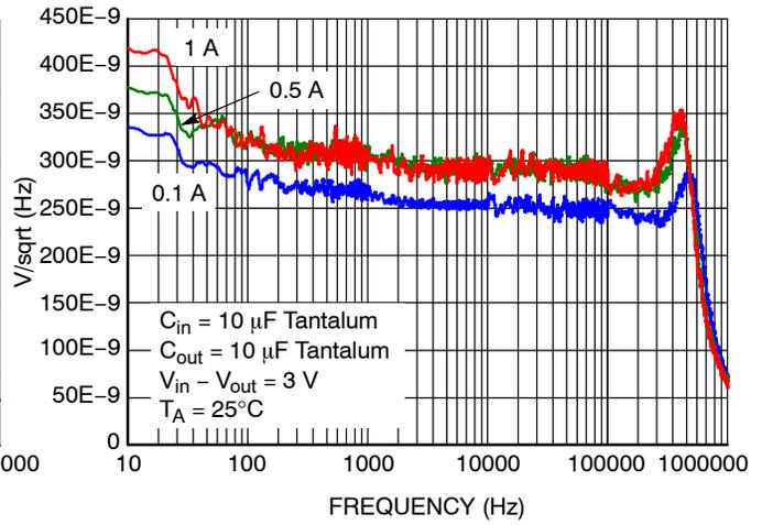
Figure 17. Output Spectral Noise Density vs. Frequency –  $V_{out} = 1V5$
