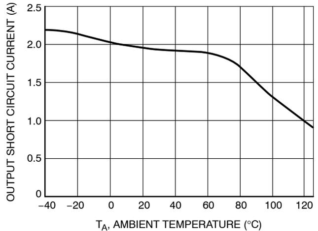
**Figure 9. Output Short Circuit Current vs. Temperature**
