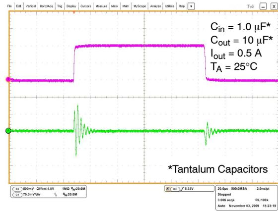
Figure 25. Line Transient Response –  $V_{out} = 3.3 V$
