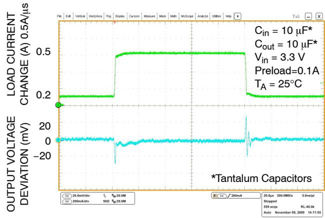
Figure 29. Load Transient Response –  $V_{out} = 2.5 V$
