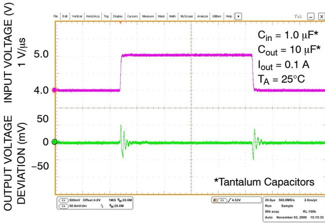
Figure 22. Line Transient Response –  $V_{out} = 2.5 V$
