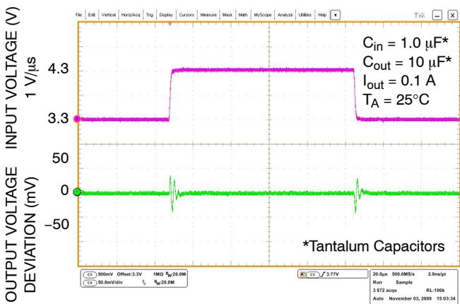
Figure 20. Line Transient Response –  $V_{out} = 1.8 V$
