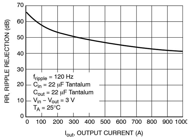
**Figure 15. Ripple Rejection vs. Output Current**
