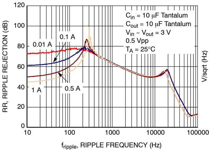
Figure 16. Ripple Rejection vs. Frequency –  $V_{out} = 1.5 V$
