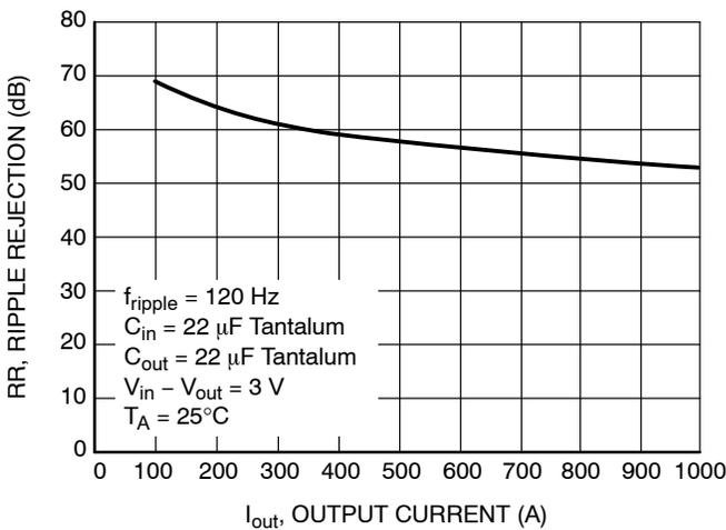
**Figure 14. Ripple Rejection vs. Output Current**
