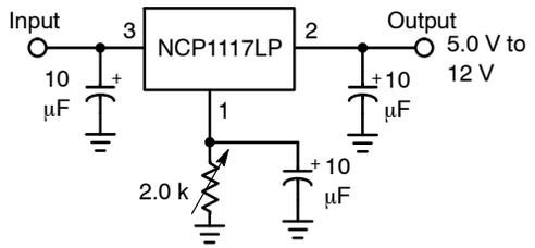
**Figure 41. Adjusting Output of Fixed Voltage Regulators**
