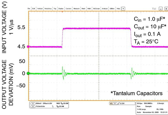
Figure 24. Line Transient Response –  $V_{out} = 3.3 V$
