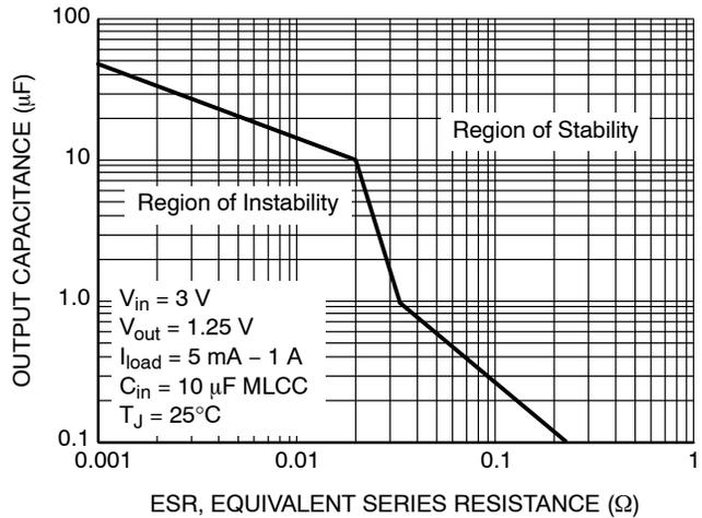
**Figure 13. Output Capacitance vs. ESR MLCC Capacitor**
