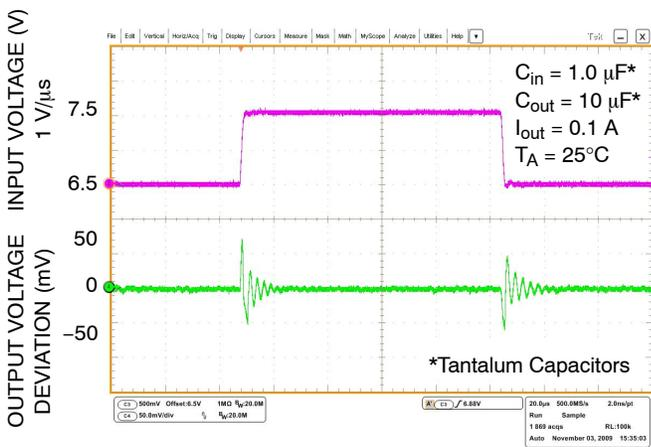
Figure 26. Line Transient Response –  $V_{out} = 5.0 V$
