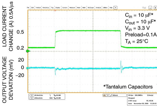
Figure 28. Load Transient Response –  $V_{out} = 1.8 V$
