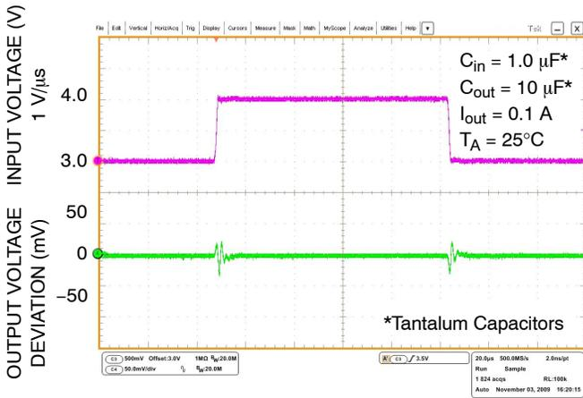
Figure 18. Line Transient Response –  $V_{out} = 1.5 V$
