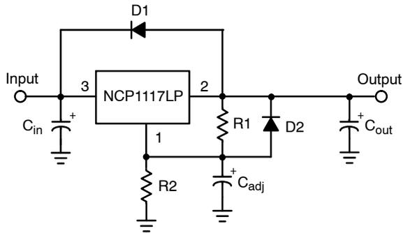
Figure 35. Protection Diode Placement
