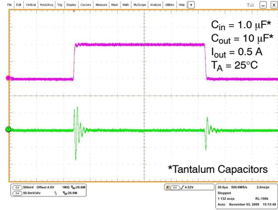
Figure 23. Line Transient Response –  $V_{out} = 2.5 V$
