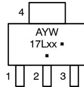
Heatsink tab is connected to Pin 2.
