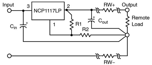
Figure 36. Load Sensing
